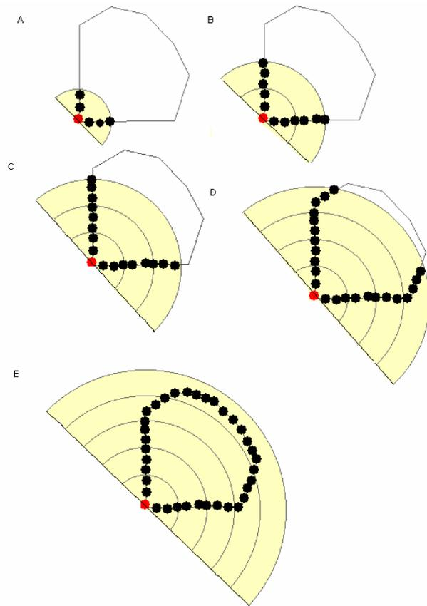
Figure 4 Sample of Circular Cast built for Irregular Building Structure from Step A to E
