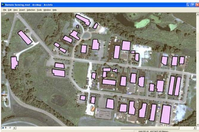
Figure 7 Extracted Buildings from the Test Area
