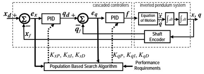
Fig. 7. Block diagram of inverted pendulum system for parameter optimization
