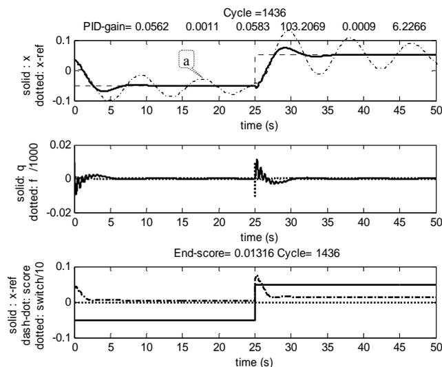
Fig. 11 Trajectory plots comparing the tracking error of (a) initial and the best scored PID parameters obtained by the real-time DE search.
