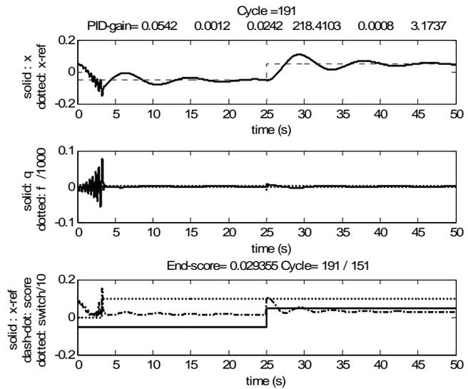
Fig. 9.b During the test of an unstable controller parameter set PID parameters were switched to  $x_s$  at  $t=2.8\text{s}$ .
