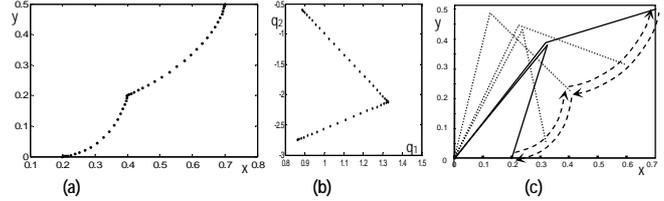
Fig. 3. Plots of the desired trajectory (a)  $x$  vs.  $y$  (in meters), (b)  $q_1$  vs.  $q_2$  (in radians), (c) the movement of the links in  $x$ - $y$  plane.
