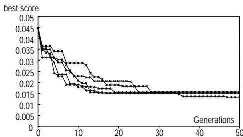
Fig. 10 Convergence-rate plots for five DE search runs with exactly the same initial parameters.
