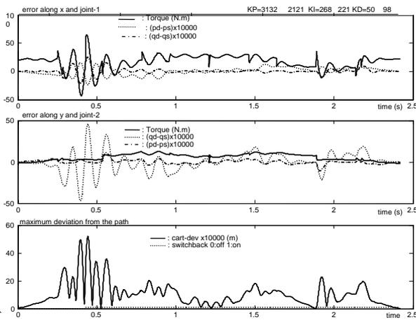
Fig. 5 b. An unstable parameter set causes excessive cartesian error at  $t=0.42$ , and control is switched back to  $x_s$ .
