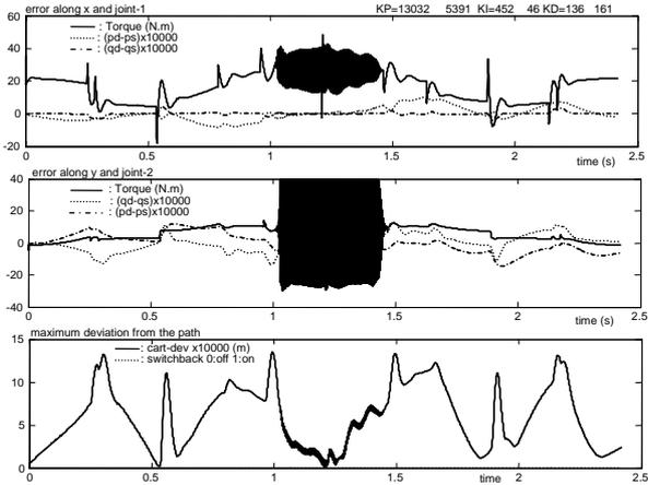
Fig. 5 c. The best parameter set reduced the cartesian error to 50%, but bounded oscillatory action of torques were observed because of the high proportional gain.
