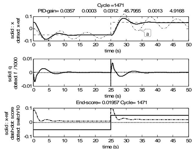
Fig 9.c Trajectory with the best scoring PID setting after 50 generations. On the first graph the trajectory (a) belongs to the initial PID settings  $x_s$ , inserted to the graph to compare initial and best-scored cases.
