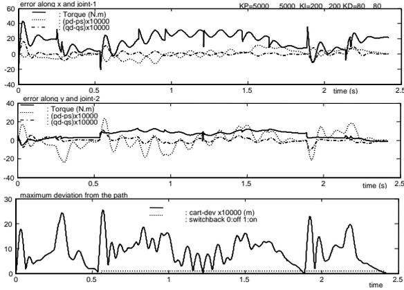
Fig. 5 a. Tracking performance of manipulator with initial stable control parameter set  $w_s$ .
