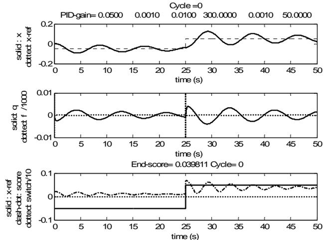
Fig. 9.a The initial stable parameter set  $x_s$  is oscillatory, but it satisfies the tracking error tolerance  $J^*$ .
