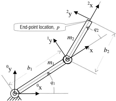
Fig. 2. Parameters of the simulated manipulator with 2-revolute joints.
