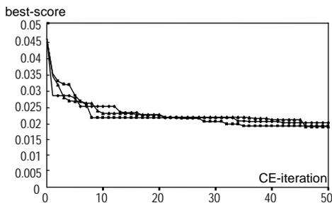
Fig. 8 Convergence-rate plots for three CE search runs with exactly the same initial parameters.
