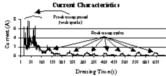
Figure 3. Current characteristics during in-process electrical dressing
