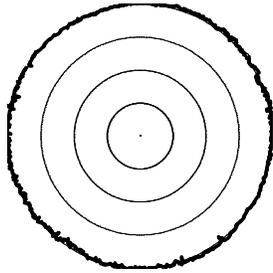
Figure 6. Wheel roundness produced by electrical dressing
