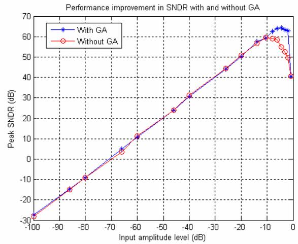
Figure 7: SNDR versus input signal amplitude with and without GA
