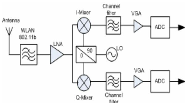
Figure 1: Zero-IF Receiver Architecture.
