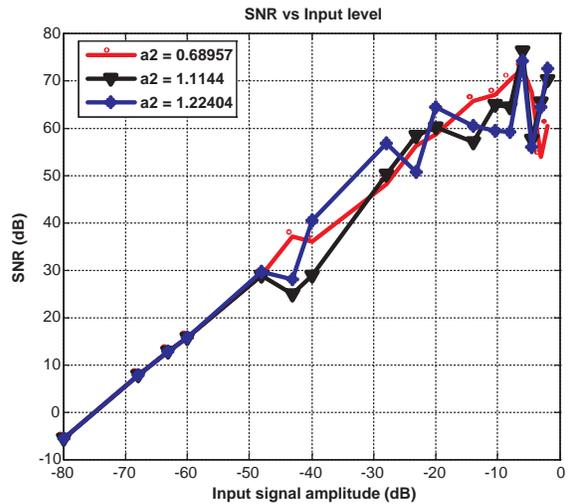
Figure 10: SNR vs. input amplitude for a second-order traditional topology
