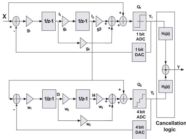
Figure 2: Modified cascaded sigma-delta modulator for WLAN
