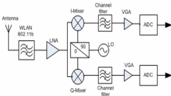
Figure 1: Zero-IF Receiver Architecture.
