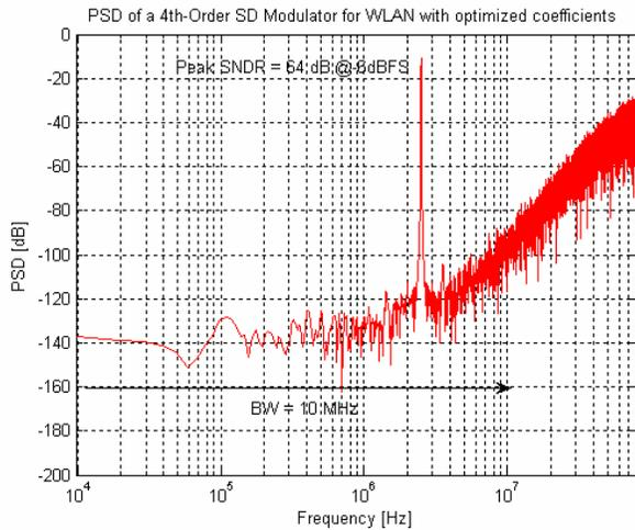
Figure 6: Modulator output spectrum for WLAN
