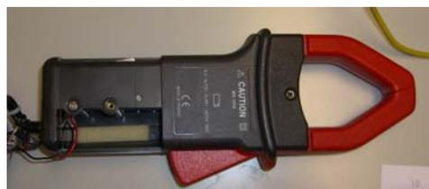
Fig. 12 – Amperimetric Clamp PAC 21 from Chauvin Arnoux.
