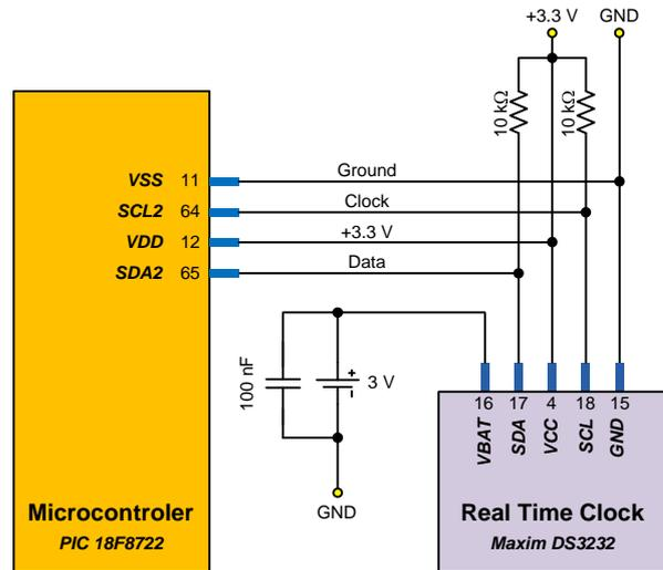
Fig. 14 – Connection diagram between the microcontroller and the real time clock.
