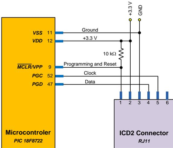
Fig. 13 – Connection diagram between the microcontroller and ICD2 debugger.
