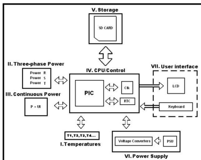
Fig. 2 – Block diagram of the measurement system.
