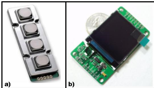
Fig. 16 – Photographs of the keypad (left) and LCD (right) used.
