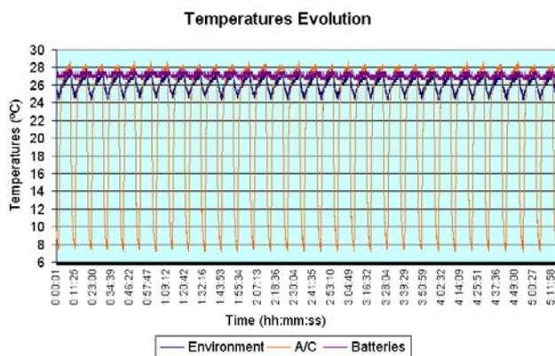
Fig. 23. Temperatures Evolution in a short period of time.
