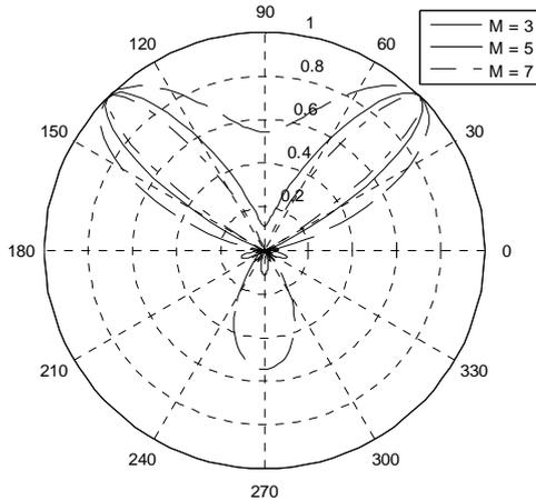
Fig. 14. Radiation pattern of the beamformer
