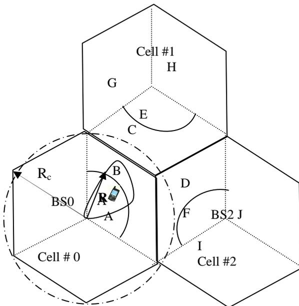
Fig.1 Cellular Layout for soft HO. A,E,F are non HO region. B,C,D are soft HO region. Cell #0 is reference cell. Adaptive transmit beamforming at BS<sub>0</sub> has been applied for the MS (shown in figure). Other users are also present (but not shown in the figure). The desired user is tracked by the specific beam during the call.
