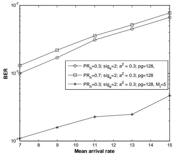
Fig. 2. Effects of beamforming and soft handoff on BER.
