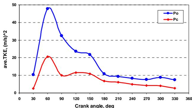
Fig.8. Variation of average TKE with crank angle positions
