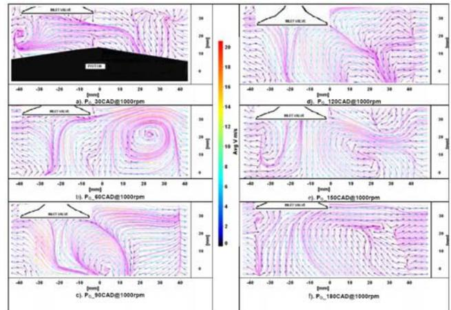
Fig.3. Ensemble average velocity vectors of pentroof with offset cavity piston during suction stroke
