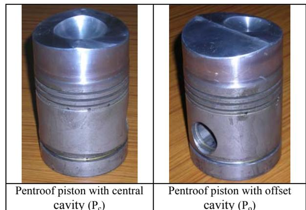
Fig.2. Pictorial view of the pentroof pistons
