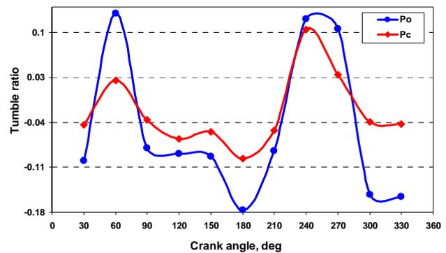
Fig.7. Variation of tumble ratio with crank angle positions
