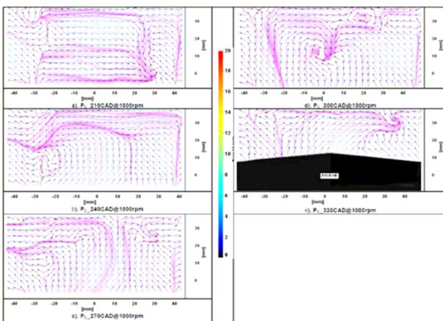
Fig.6. Ensemble average velocity vectors of pentroof with central cavity piston during compression stroke
