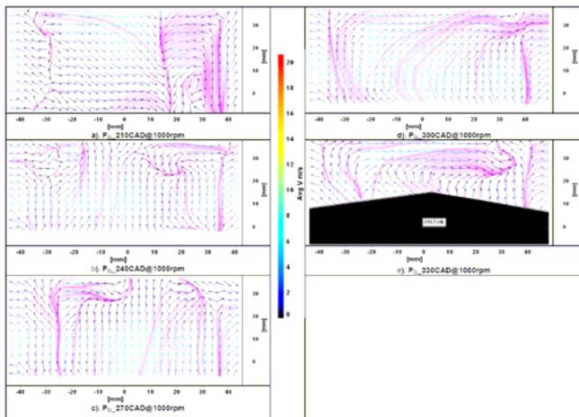
Fig.5. Ensemble average velocity vectors of pentroof with offset cavity piston during suction stroke
