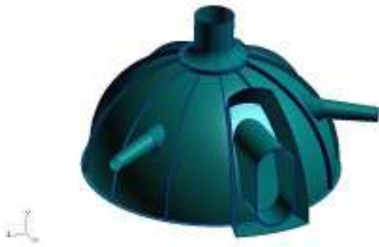
Fig. 1. Large underground spherical cap shelter made from thin sandwich composite structures
