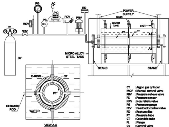
Figure 4: Schematic of the Test Setup for ballooning experiment.
