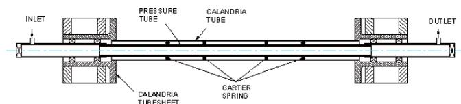
Figure 1: Schematic of Indian PHWR Reactor Channel
