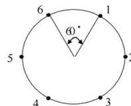
Figure 3: Circumferential thermocouples positions at any axial location
