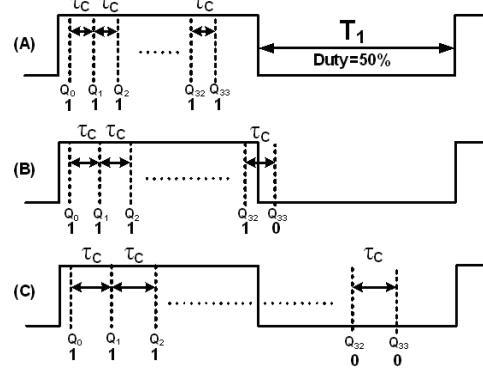
Fig. 5 Cyclic time detector lock-in diagram
