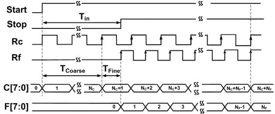
Fig. 9 Time diagram of the proposed TDC
