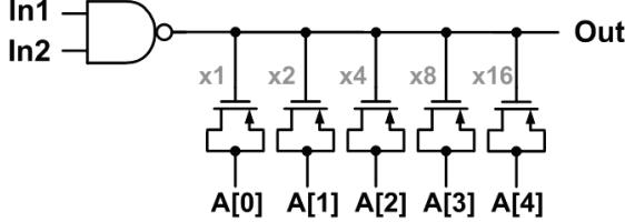
Fig. 3 Digital control delay element
