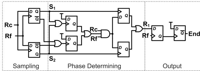
Fig. 7 Proposed phase coincidence detector Circuit
