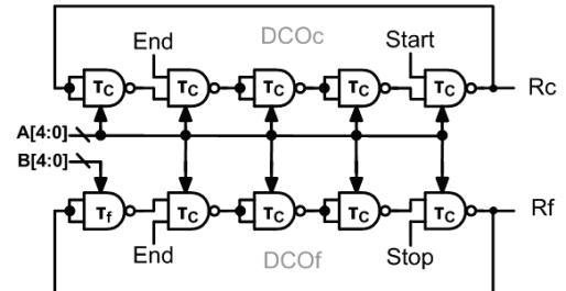
Fig. 6 Proposed digital control oscillator circuit
