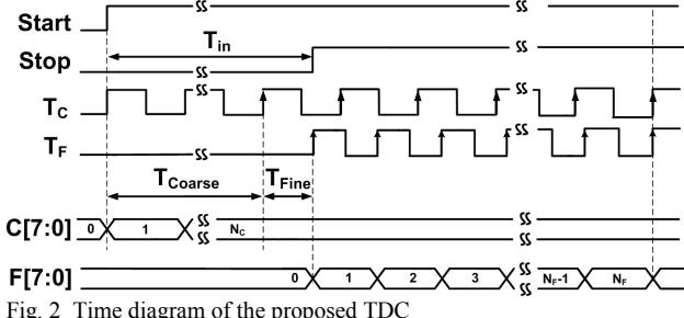
Fig. 2 Time diagram of the proposed TDC
