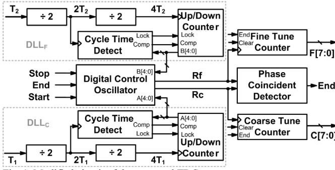
Fig. 1 Modified circuit of the proposed TDC
