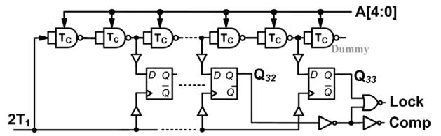
Fig. 4 Circuit of the cyclic time detector
