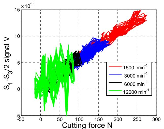
Fig. 5. The relation between the spindle displacements and cutting forces at different spindle speeds.
