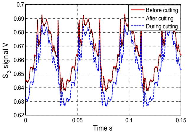
(b) The output of the  $S_3$  sensor signals
