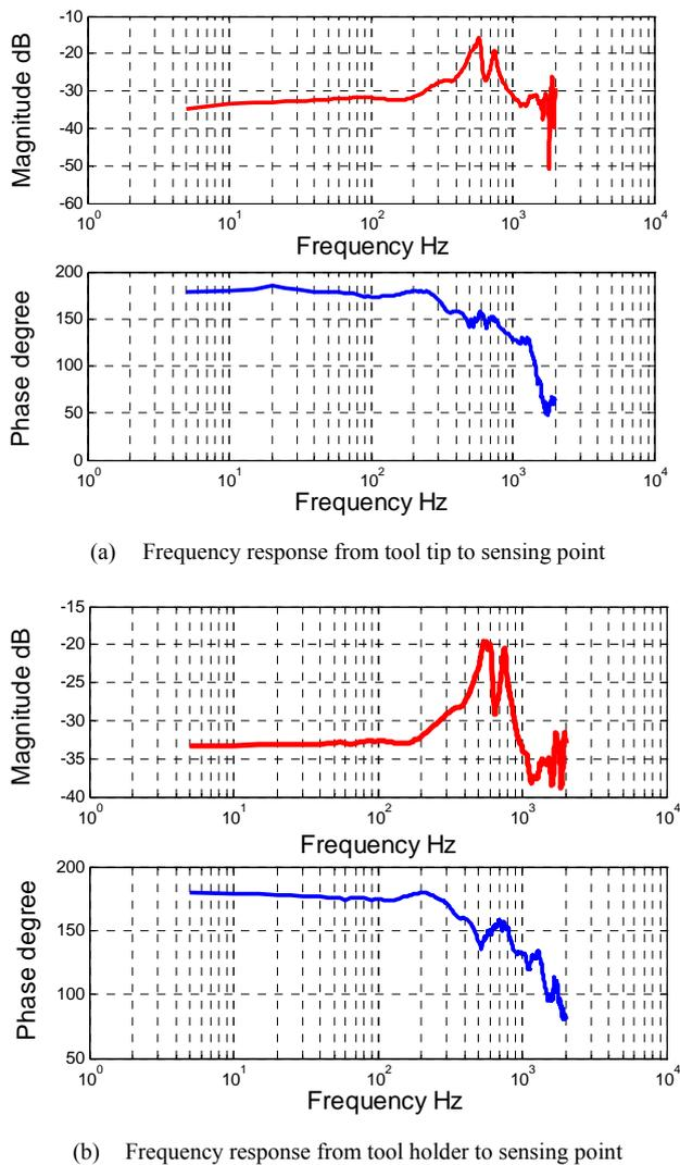
Fig. 6 Frequency response of displacement sensor  $S_3$
