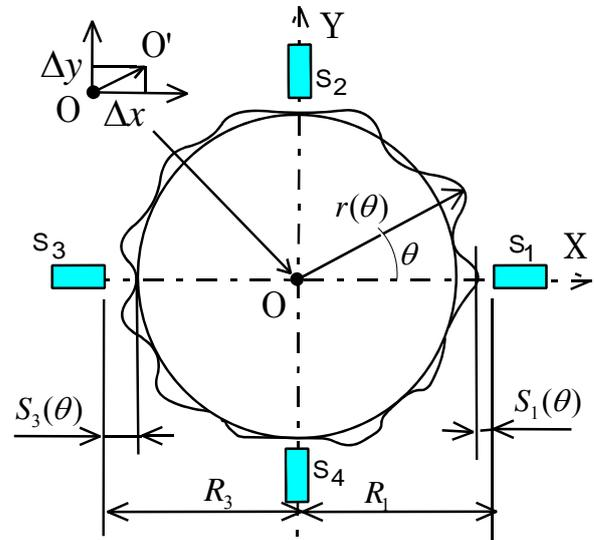
Fig.3. The concept of the spindle displacement measurement
