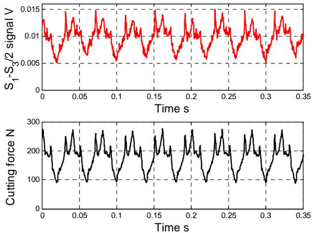
(a) Spindle speed: 1500 min<sup>-1</sup>
