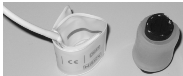
Fig. 3. Cuff and bung for measuring light transmission through a sheep ear during occlusion.
