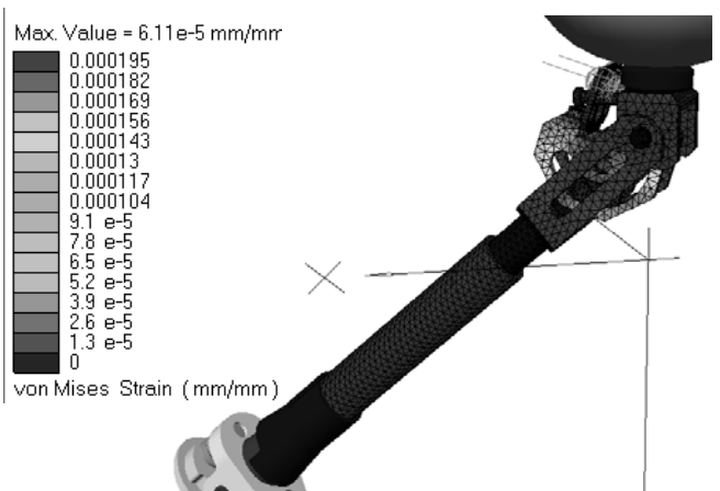
Fig. 28. Deformations of the parameterized knee prosthesis
