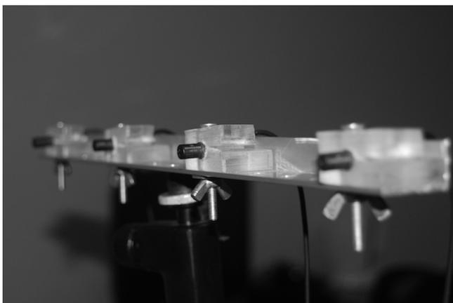
Fig. 4. The four-microphone, 1-D beamformer during the experiments. The devices is a part of Automatic Speech Recognition system.
