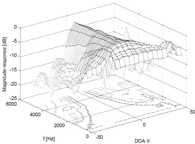
Fig. 3. Results of the iterative optimization of beamformer in adverse acoustic environment having the desired system response.
