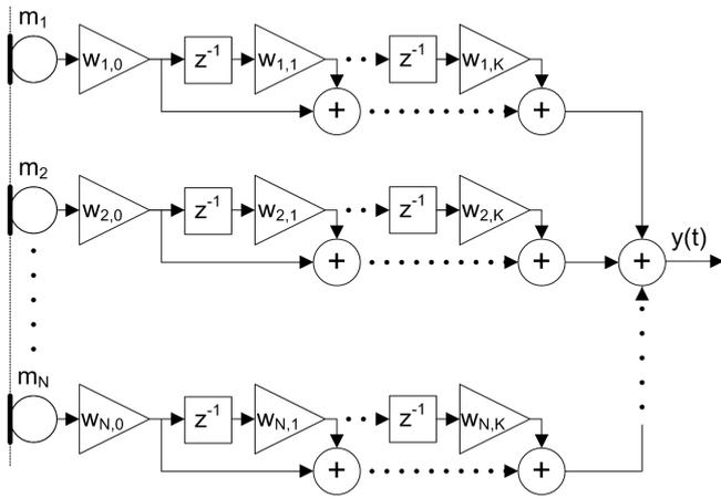
Fig. 1. A general structure of filter-and-sum beamformer.
