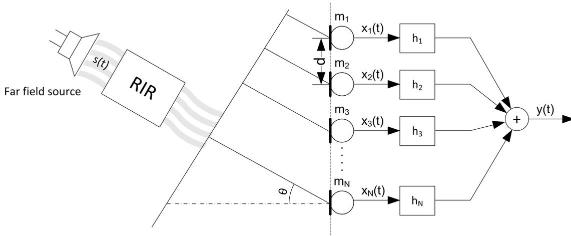
Fig. 2. 1-D beamformer placed in acoustic environment with far field source modified by RIR.
