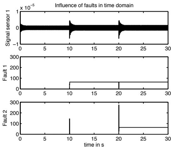
Fig. 8. Observed fault amplitude by means of augmented observer
