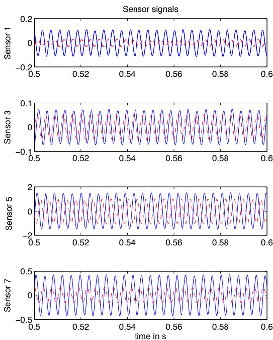
Fig. 5. Measured sensor signals, solid line: sensor signals without fault, dashed line: sensor signals with fault
