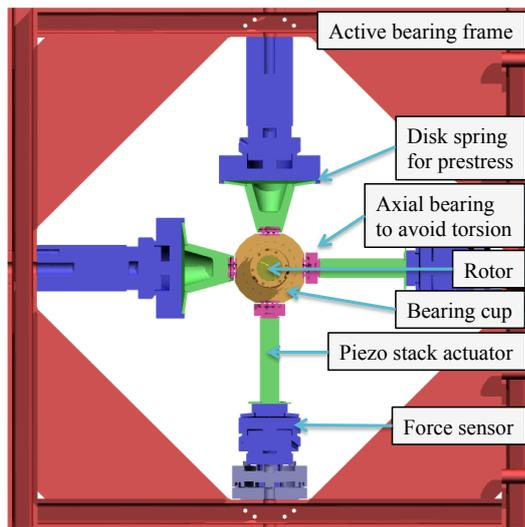
Fig. 3. Active bearing configuration
