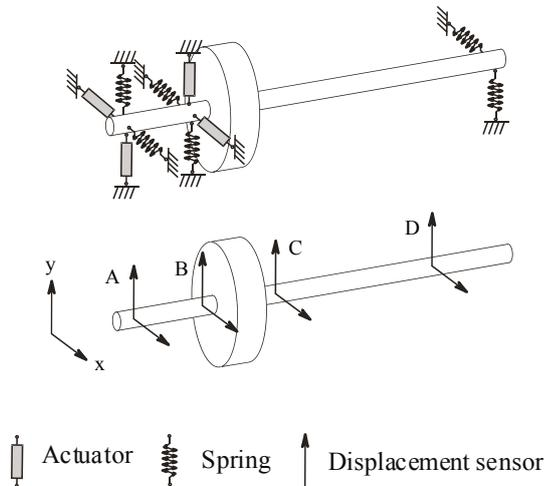
Fig. 7. Configuration of the rotor test rig
