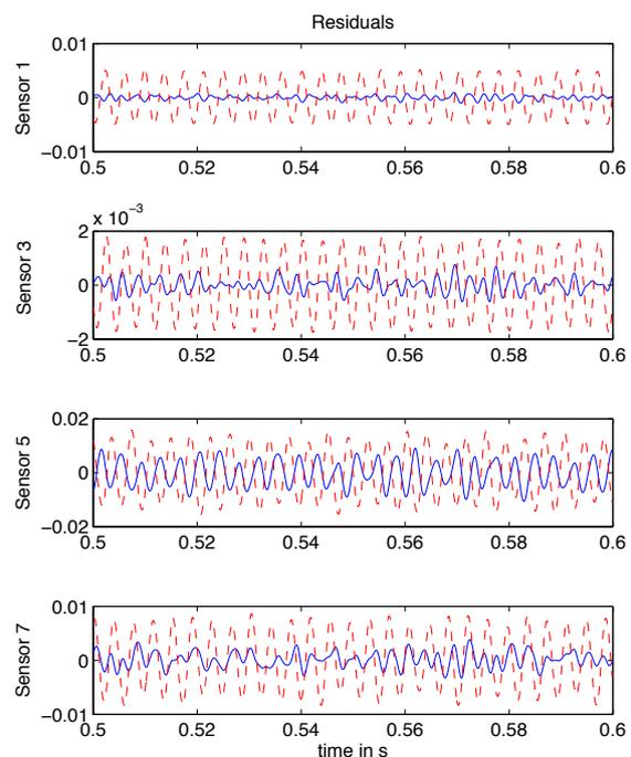
Fig. 6. Residuals generated by augmented observer, solid line: residuals without fault, dashed line: residuals with fault
