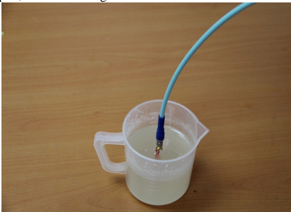
Fig. 21. The antenna placed in the liquid
