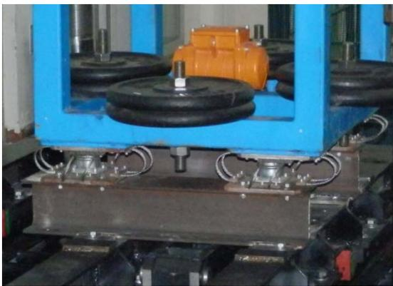
Fig. 16. Cabinet isolators and additional masses.
