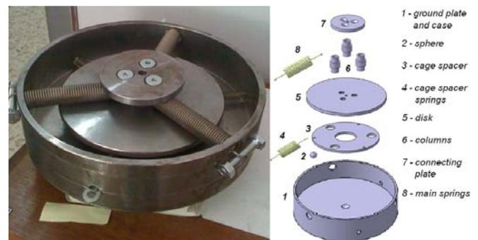
Fig. 1. Rolling seismic isolator with helical springs (DII, Naples, Italy).
