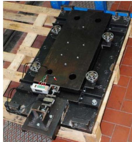
Fig. 9. Device for the characterization of isolator stiffness.
