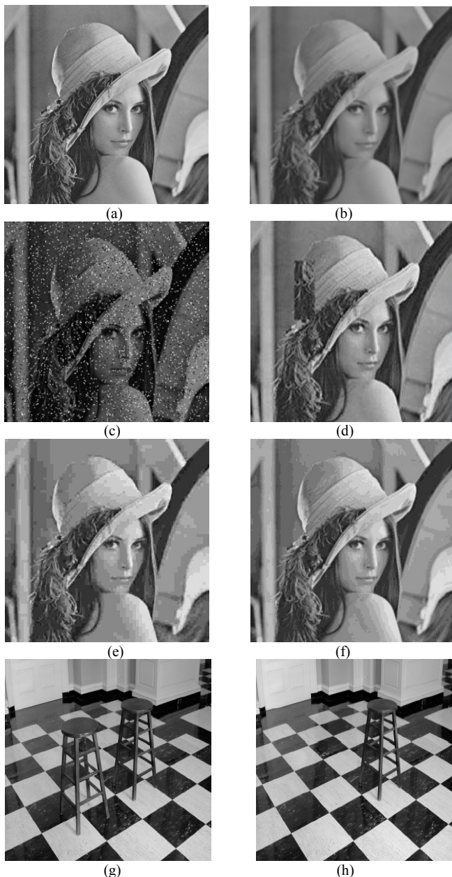
Fig. 1. Different types of attacks (a) Authentic image (b) Gaussian blurring (c) Noise Addition (AWGN) (d) Copy-Move attack (e) JPEG Compression at ratio 32:1 (f) JPEG Compression at ratio 20:1 (g) Authentic Image (h) Image Splicing
