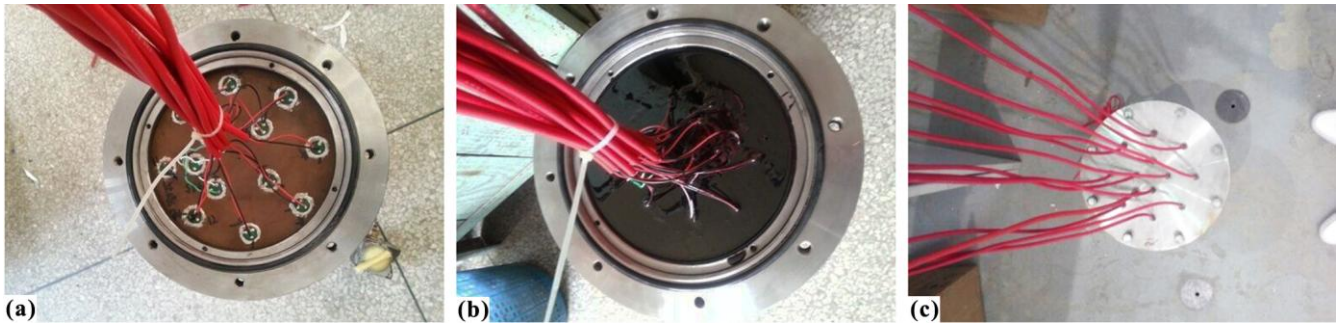
Fig. 3. Data acquisition unit waterproof sealing (a- Data acquisition unit; b- Interior waterproof; c- Exterior waterproof)
