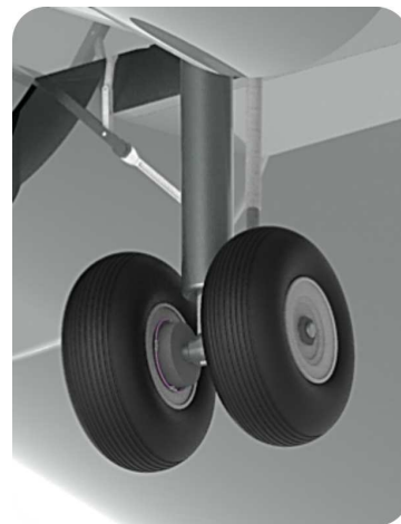
Fig. 9. Example of the simplified model of the landing gear of the Boeing 737 aircraft realized and rendered in CAD environment.
