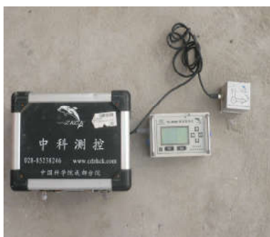
Fig. 1. Blasting vibration monitoring system
