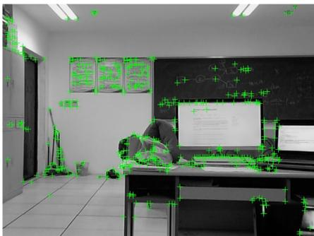
Fig.11. Extracted feature points of left camera at 0s
