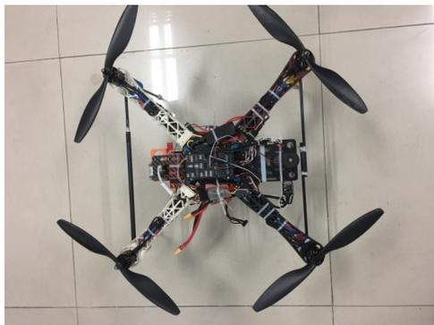
Fig.5. The UAV for our experiments
