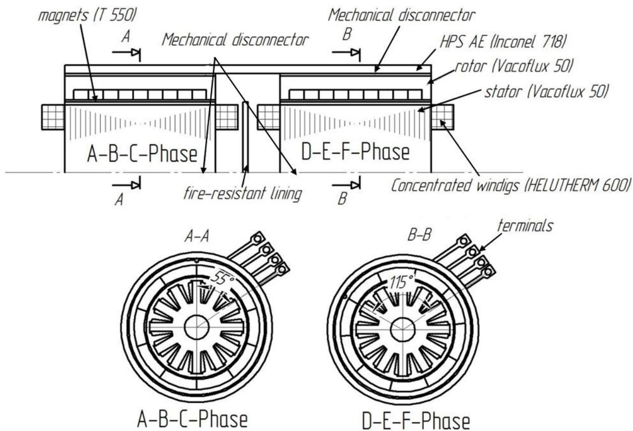
Fig. 3. Six-Phase high temperature SG embedded on the HPS
