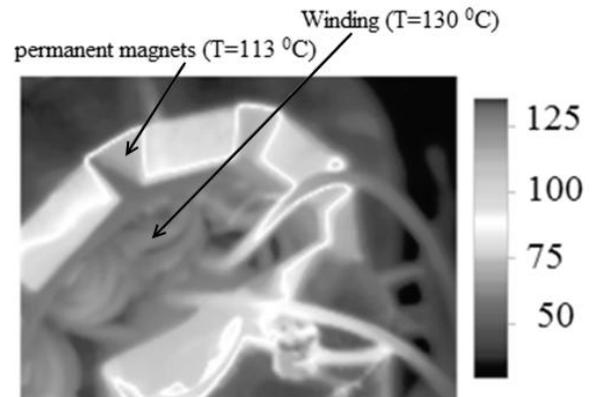
SG thermal image after heating for 1 hour at 217 °C
