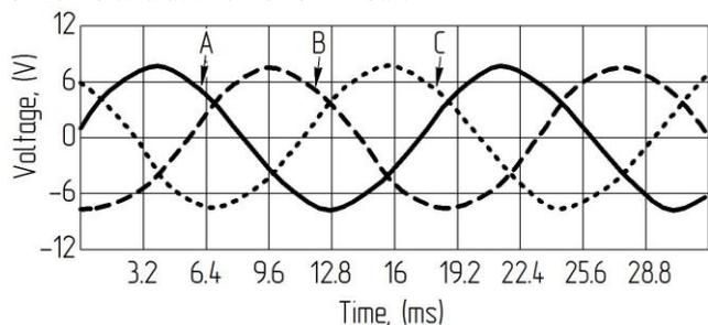
Fig. 5. Output voltage waveforms of the experimental prototype at idle and an ambient temperature of 25 °C
