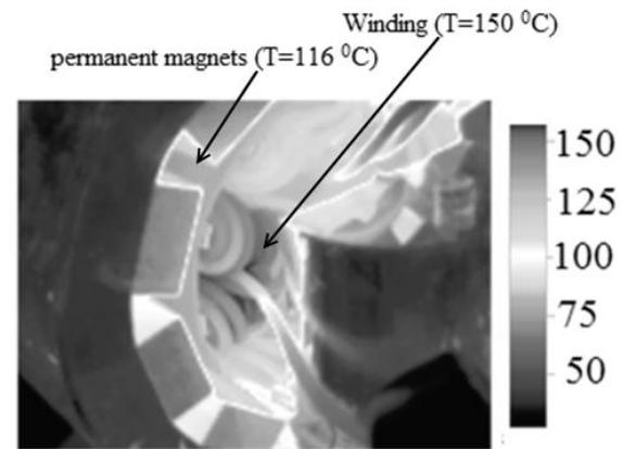
SG thermal image after heating for 1 hour at 217 °C and 40 sec of operation in the short circuit mode
