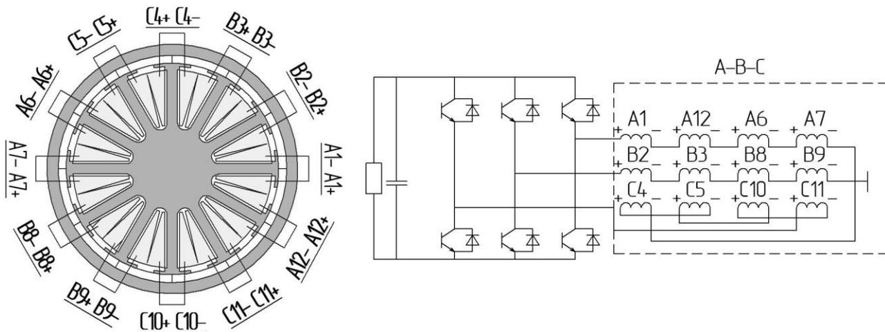
Fig. 2. High-temperature SG with external rotor and tooth-coil winding
