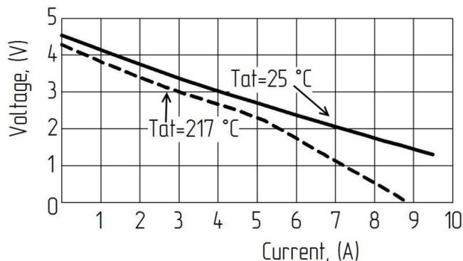
Fig. 7. Voltage and current dependencies at ambient temperature of 25 °C and at 217 °C for 1 hour
