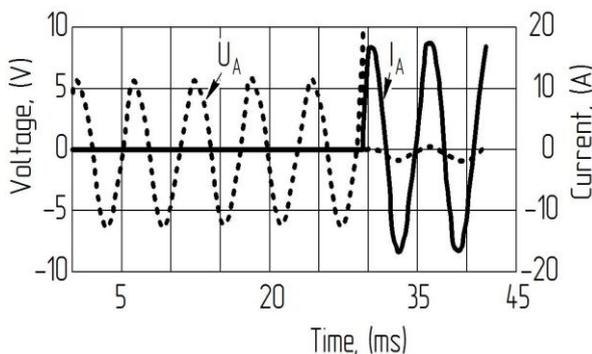
Fig. 9 Waveforms of currents and voltages at the sudden three-phase short circuit in SG
