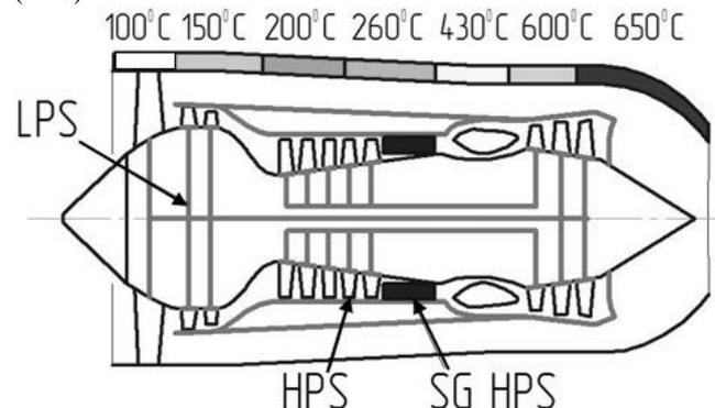
Fig. 1. Sketch of a double-shaft AE with integrated SG
