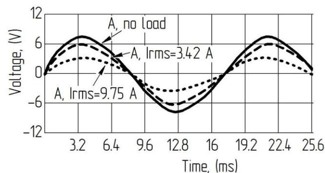
Fig. 6. Output voltage waveforms of the experimental prototype at various loads and an ambient temperature of 25 °C
