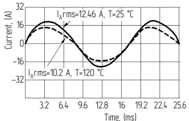
Fig. 11. Waveforms of sudden single-phase short circuit current in SG at different temperatures
