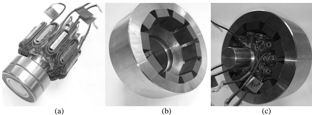
Fig. 4. (a) – stator of the experimental model; (b) – rotor of the experimental model; (c) – assembled experimental model
