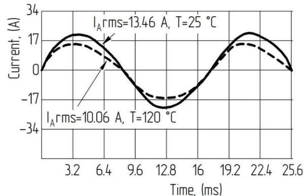
Fig. 10. Waveforms of sudden three-phase short circuit currents in SG at different temperatures
