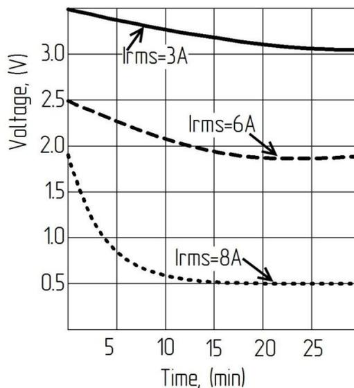
Fig. 8. Power characteristics curves of the experimental SG prototype
