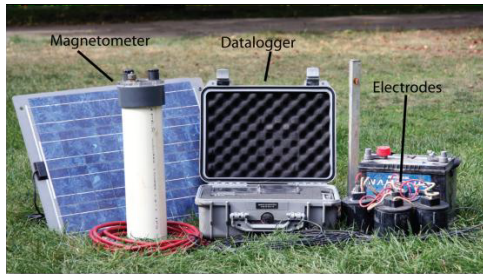
Fig. 2: Typical MT equipment (from Nieuwenhuis, 2011[6]).
