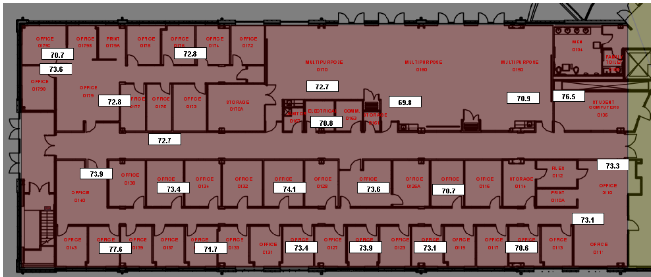
Fig. 2. A temperature map collected by distributed sensors in an office building captured from a BAS of Johnson Controls
