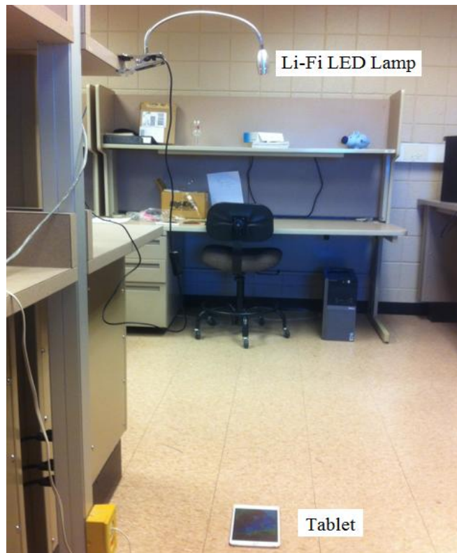
Figure 7. Li-Fi communication setups in an office building [35] (this figure is owned by me)
