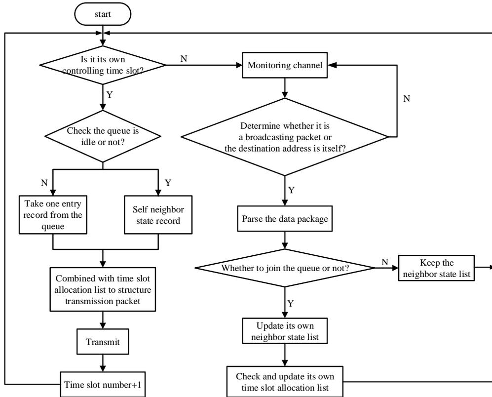
Fig. 4. Interaction process of the TDMA protocol.
