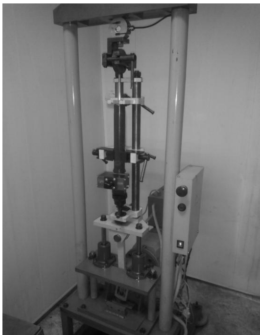
Fig. 7. Experimental stand for the shock absorber test
