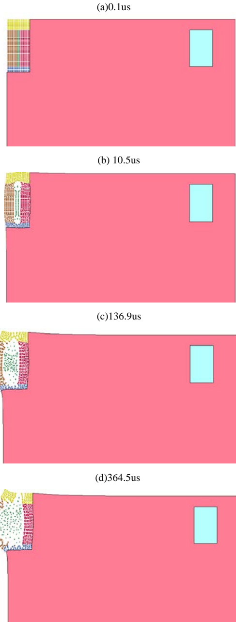
Fig. 3. The deformation of near zone under the deep hole bench blasting
