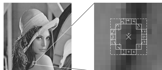
Fig. 2. An example of the segment test
