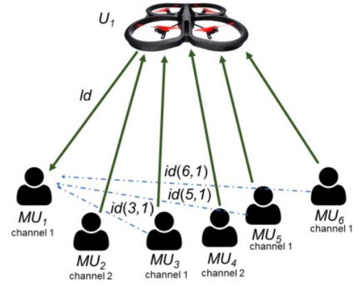
Fig. 3: Calculation of the SIR in a mobile user
