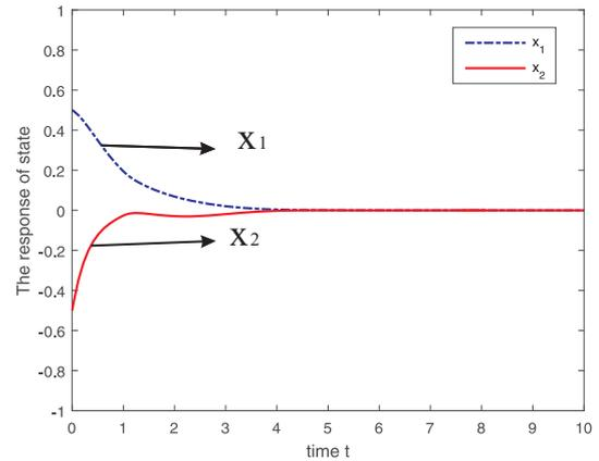
Fig. 3: State response of the subsystem 1.
