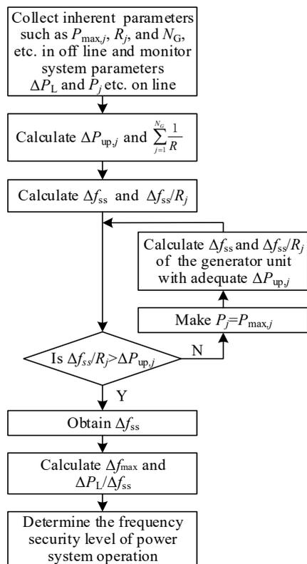
Fig.3 Flow-chart of the frequency security level grading of power system operation.
