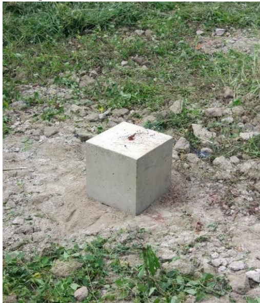
Fig. 11 Cubic concrete with a borehole at the centre of the top surface
