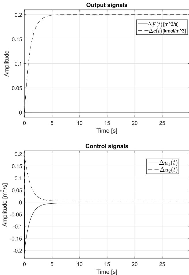
Fig. 4. Control signals and stirred tank output signals to  $\Delta F(t) = 0$  and  $\Delta c(t) = 0.2$  reference signals.
