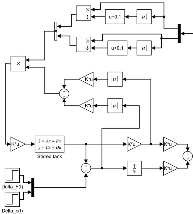
Fig. 2. Stirred tank using Simulink.
