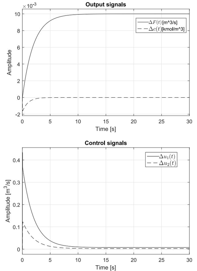
Fig. 3. Control signals and stirred tank output signals to  $\Delta F(t) = 0.01$  and  $\Delta c(t) = 0$  reference signals.
