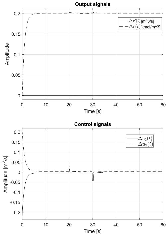
Fig. 8. Control signals and stirred tank output signals to  $\Delta F(t) = 0$  and  $\Delta c(t) = 0.2$  reference signals and step disturbances.
