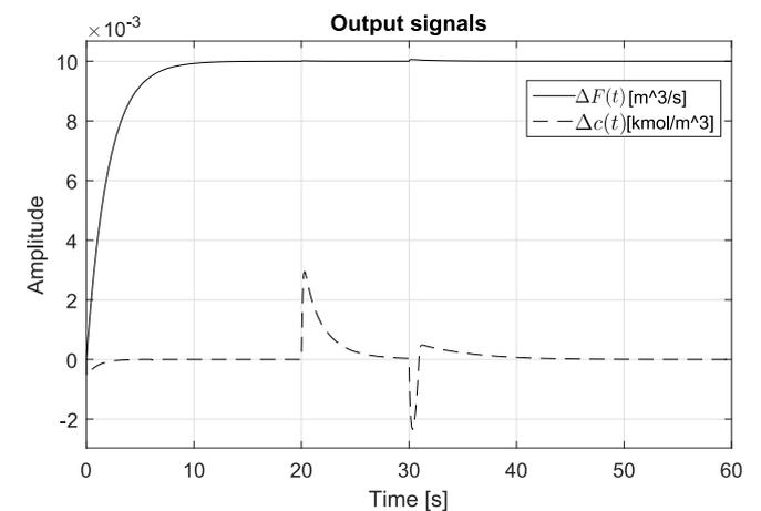
Fig. 7. Control signals and stirred tank output signals to  $\Delta F(t) = 0.01$  and  $\Delta c(t) = 0$  reference signals and step disturbances.
