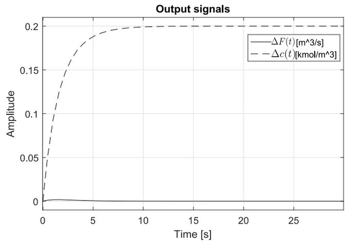
Fig. 6. Stirred tank output signals to  $\Delta F(t) = 0$  and  $\Delta c(t) = 0.2$  reference signals.
