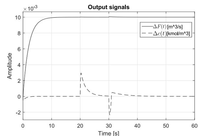
Fig. 7. Control signals and stirred tank output signals to  $\Delta F(t) = 0.01$  and  $\Delta c(t) = 0$  reference signals and step disturbances.
