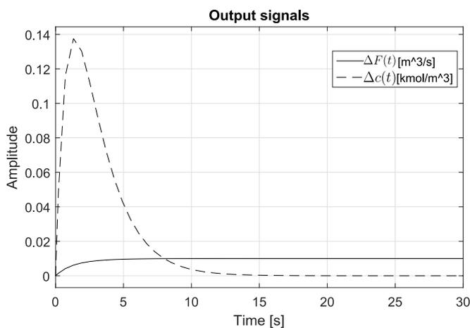
Fig. 5. Stirred tank output signals to  $\Delta F(t) = 0.01$  and  $\Delta c(t) = 0$  reference signals.
