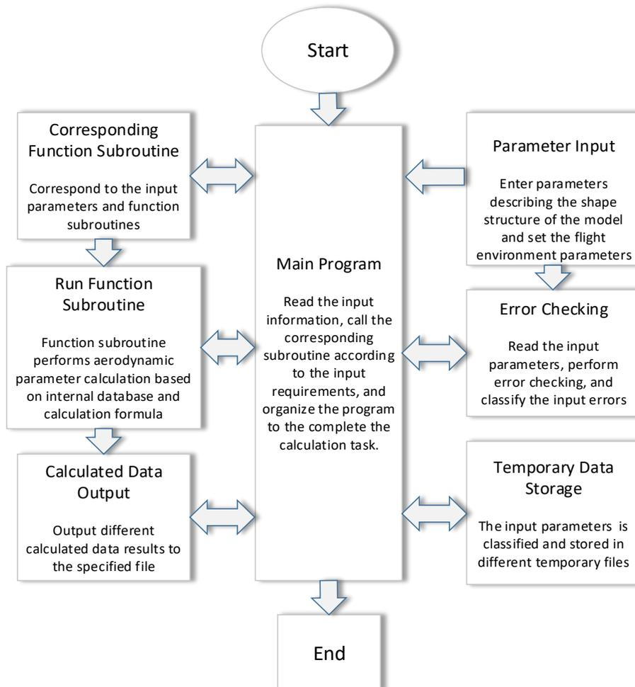
Fig. 1. DATCOM running process
