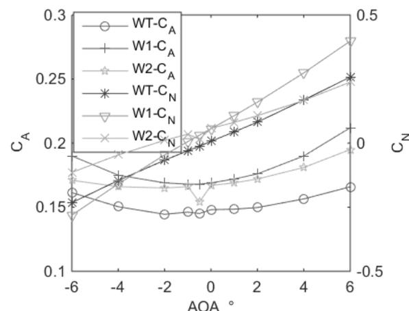
Fig. 4.  $C_A$ -AOA &  $C_N$ -AOA at 0.8 Mach
