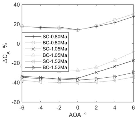
Fig. 10 Error of  $C_A$  varies with the AOA
