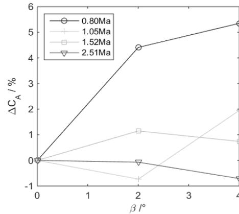
Fig. 21. The variation of  $C_A$  error with the  $\beta$  after compensation correction
