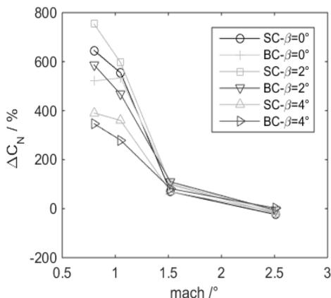
Fig. 23 Variation of  $C_N$  error with Mach numbers at different  $\beta$
