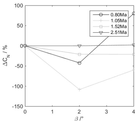
Fig. 24. The variation of  $C_N$  error with the  $\beta$  after compensation correction
