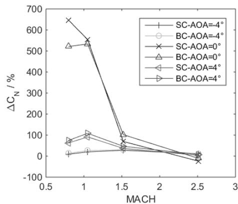
Fig. 13 Error of  $C_N$  varies with the Mach
