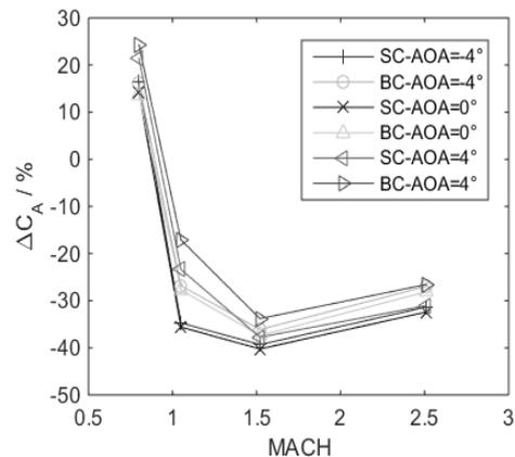
Fig. 9 Error of  $C_A$  varies with the Mach
