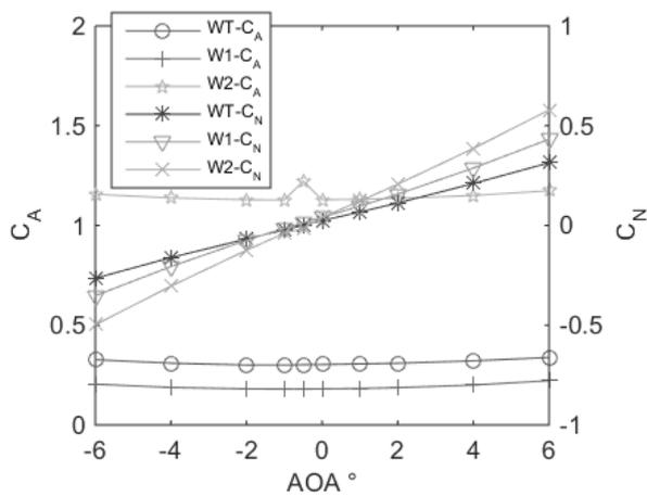
Fig. 6.  $C_A$ -AOA &  $C_N$ -AOA at 1.52 Mach
