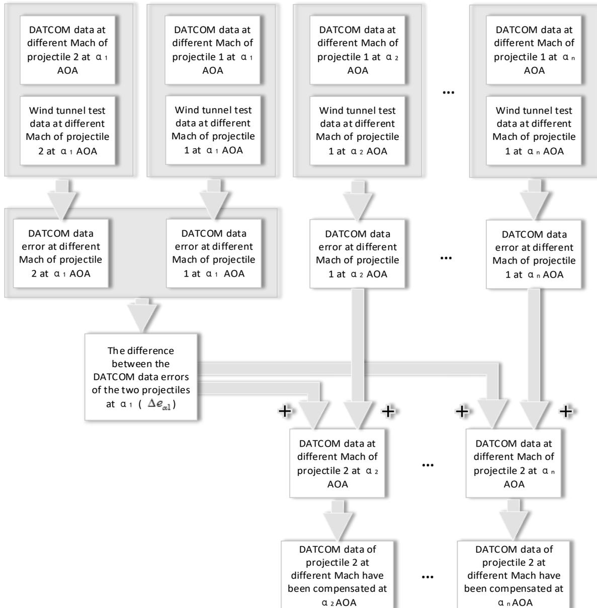
Fig. 11. Implementation process of the SECM
