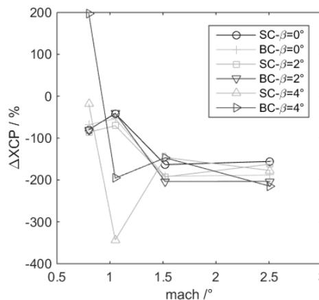
Fig. 26 Variation of XCP error with Mach numbers at different  $\beta$
