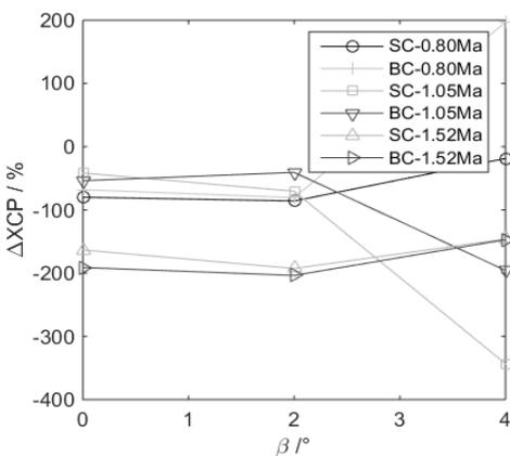
Fig. 25 Variation of XCP error with  $\beta$  at different Mach Numbers
