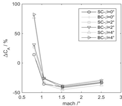
Fig. 20 Variation of  $C_A$  error with Mach numbers at different  $\beta$
