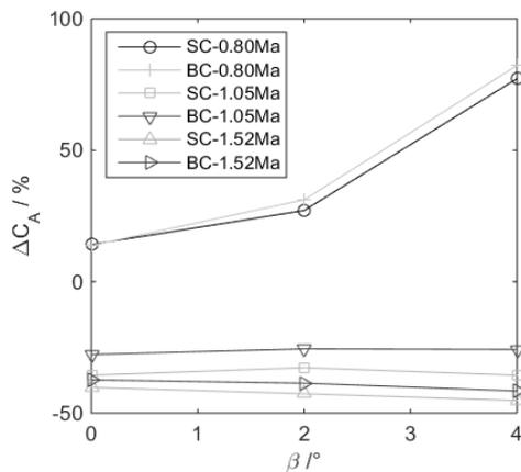
Fig. 19 Variation of  $C_A$  error with  $\beta$  at different Mach Numbers
