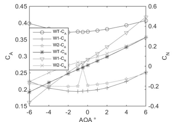
Fig. 5.  $C_A$ -AOA &  $C_N$ -AOA at 1.15 Mach
