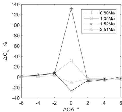
Fig. 15  $C_N$  error of big canard projectile after compensation correction
