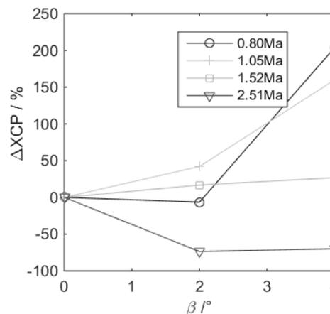
Fig. 27 Variation of XCP error with Mach numbers at different  $\beta$
