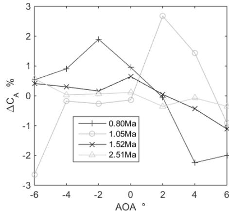
Fig. 12  $C_A$  error of big canard projectile after compensation correction
