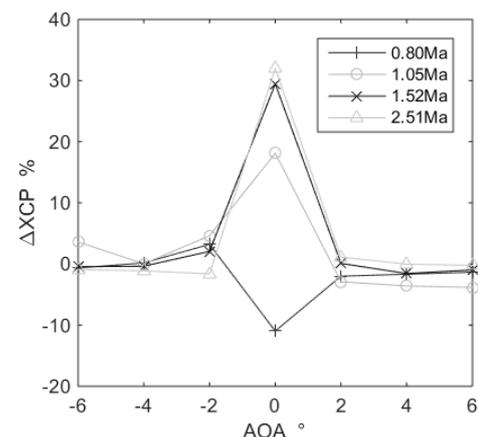
Fig. 18 XCP error of big canard projectile after compensation correction
