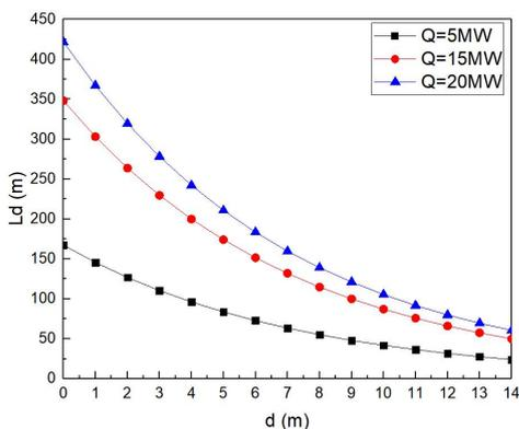
Fig. 3. The influence of heat release rate of fire.
