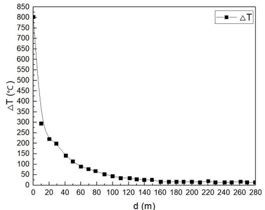
Fig. 6. Average temperature difference in fire source.
