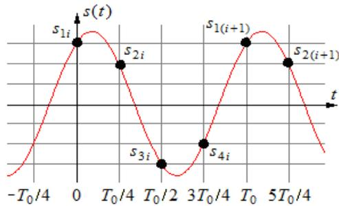
Fig. 1. Time diagram of the DPSK signal sampling.
