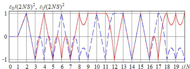
Fig. 4. The time diagrams of the demodulator responses in the absence of interferences:  $z_0/(2NS)^2$  – solid line;  $z_1/(2NS)^2$  – dashed line.
