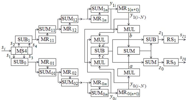
Fig. 2. The block diagram of the demodulator.
