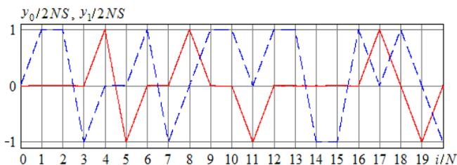
Fig. 3. The time diagrams of the quadrature channel responses in the absence of interferences:  $y_0/2NS$  – solid line;  $y_1/2NS$  – dashed line.
