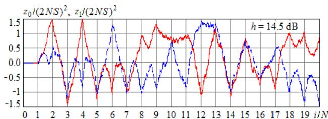
Fig. 5. Time diagrams of the demodulator responses when receiving the signal against band Gaussian noise:  $z_0/(2NS)^2$  – solid line;  $z_1/(2NS)^2$  – dashed line.
