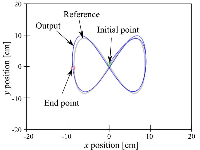
Fig. 9. System response for a trajectory tracking in simulation for  $x$ -axis and  $y$ -axis considering a bi-hemispheric cerebellum based controller.
