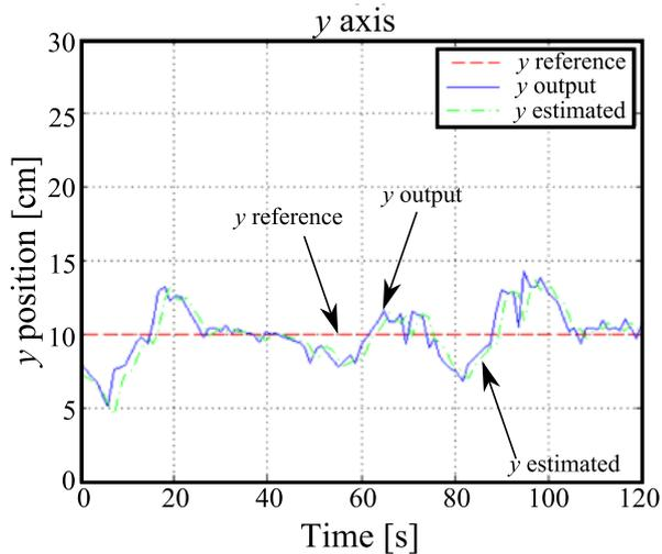
Fig. 11. System response in real time for  $y$ -axis considering a bi-hemispheric cerebellum based controller.
