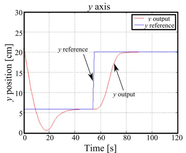
Fig. 6. Tracking response for a bi-hemispherical controller based on the cerebellum with the polynomial controller for the  $y$ -axis.
