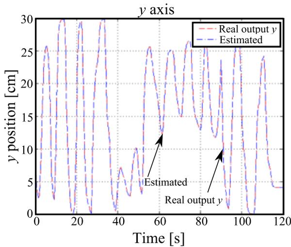
Fig. 4. Estimated and real output for  $y$  axis.
