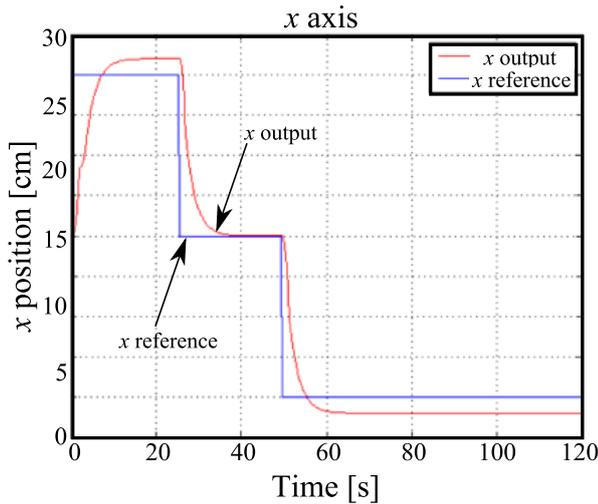
Fig. 7. Tracking response by using state feedback controller based on an extended feedback linearization method in the  $x$ -axis.
