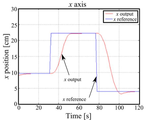
Fig. 5. Tracking response for a bi-hemispherical controller based on the cerebellum with the polynomial controller for the  $x$ -axis.
