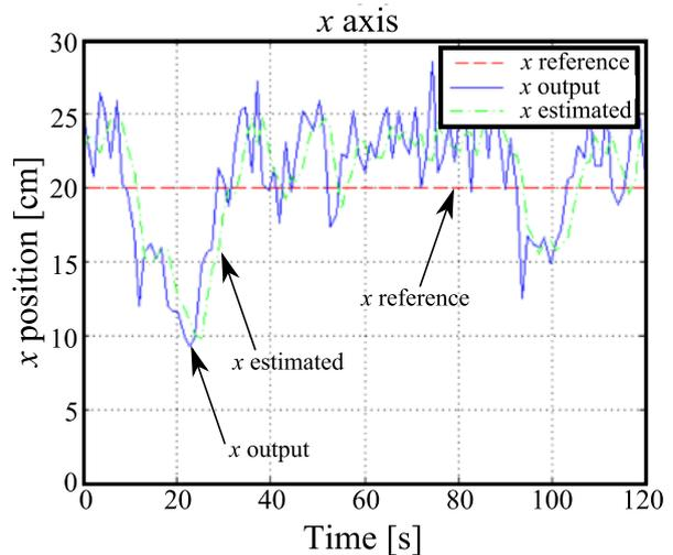
Fig. 10. System response in real time for  $x$ -axis considering a bi-hemispheric cerebellum based controller.
