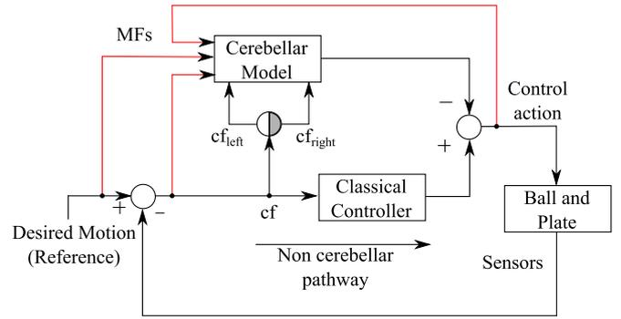
Fig. 2. Control diagram based on a bi-hemispheric cerebellum structure
