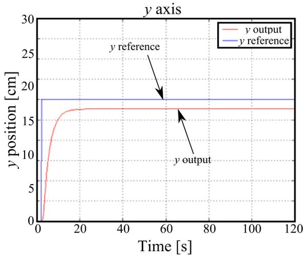
Fig. 8. Tracking response by using state feedback controller based on an extended feedback linearization method in the  $y$ -axis.
