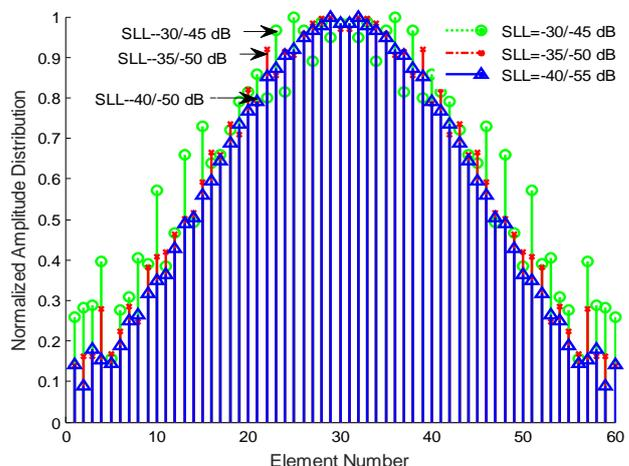
Fig. 4. Element amplitude weights obtained by APSO method for N=60, SLL=-30/-45dB, SLL=-35/-50dB, and SLL=-40/-55dB.
