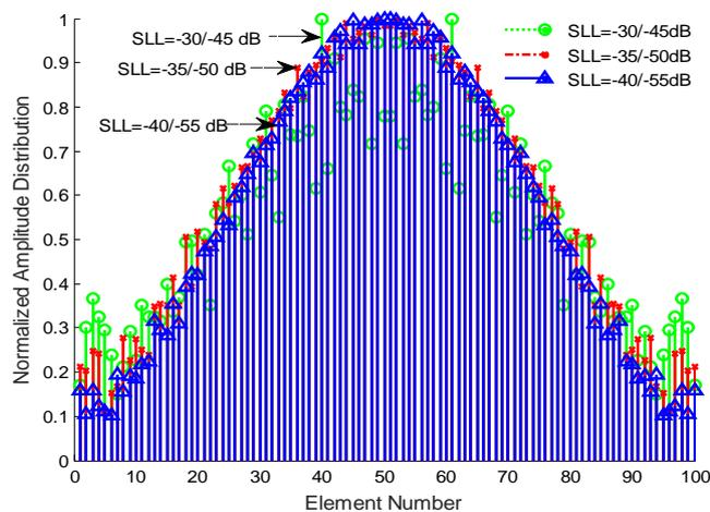
Fig. 6. Element amplitude weights obtained by APSO method for N=100, SLL= -30/-45dB, SLL=-35/-50dB, and SLL= -40/-55dB.
