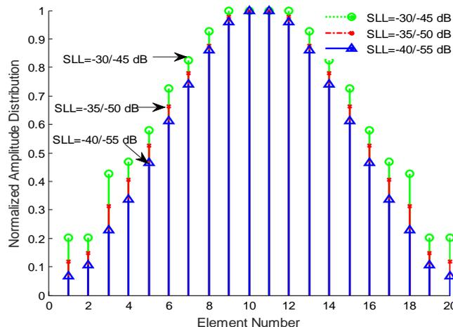
Fig. 2. Element amplitude weights obtained by APSO method for N=20, SLL=-30/-45dB, SLL=-35/-50dB, and SLL=-40/-55dB.
