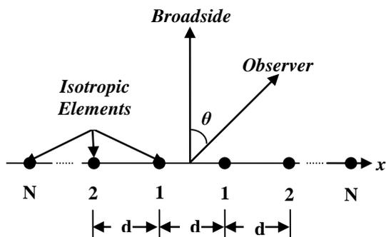
Fig. 1. Geometry of Linear Array with equal spacing.
