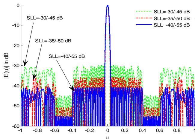
Fig. 7. Optimized Sum Pattern by APSO method for N=100, SLL=-30/-45dB, SLL=-35/-50dB, and SLL=-40/-55dB.
