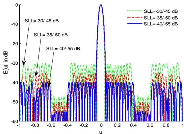
Fig. 5. Optimized Sum Pattern by APSO method for N=60, SLL= -30/-45dB, SLL=-35/-50dB, and SLL= -40/-55dB.
