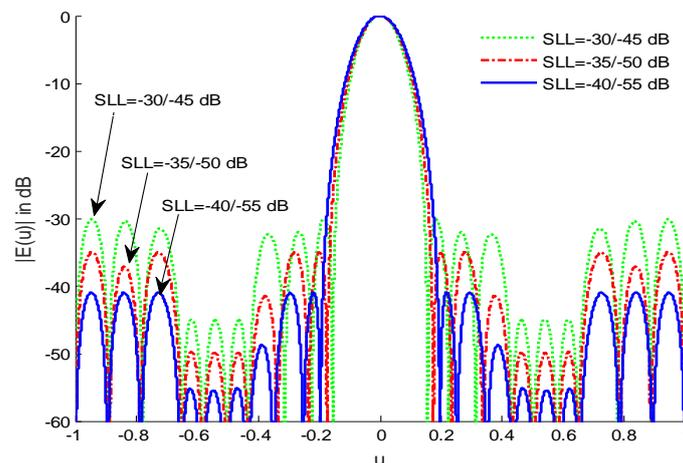
Fig. 3. Optimized Sum Pattern by APSO method for N=20, SLL=-30/-45dB, SLL=-35/-50dB, and SLL=-40/-55dB.
