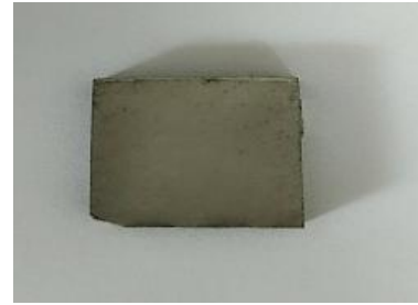
Fig. 3. Co-W film, the surface of PCrNi 3 MoVA steel surface.
