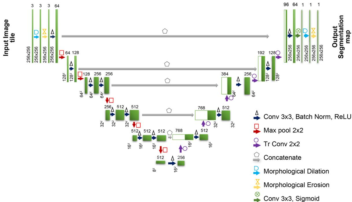
Fig. 6: Morpho-U-Net, the proposed segmentation autoencoder architecture with morphological layers at both ends.
