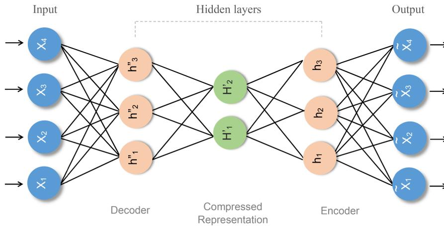
Fig. 5: A typical autoencoder architecture showing the input, hidden, and output layers.
