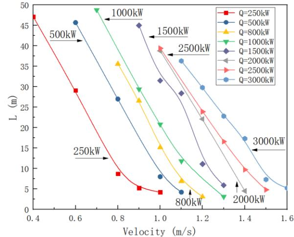
Fig. 4. The smoke back-layering length the utility tunnel with fire located at side A.
