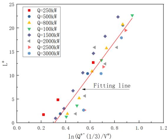
Fig. 6. Correlation of dimensionless smoke back-layering length with variable of  $\ln(Q^{*1/3}/V^*)$  when fire source at center line C location.
