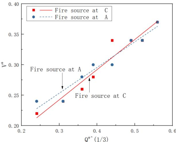
Fig. 5. The dimensionless critical ventilation velocity in the utility tunnel.
