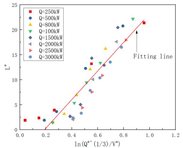
Fig. 7. Correlation of dimensionless smoke back-layering length with variable of  $\ln(Q^{*1/3}/V^*)$  when fire source located at side A.
