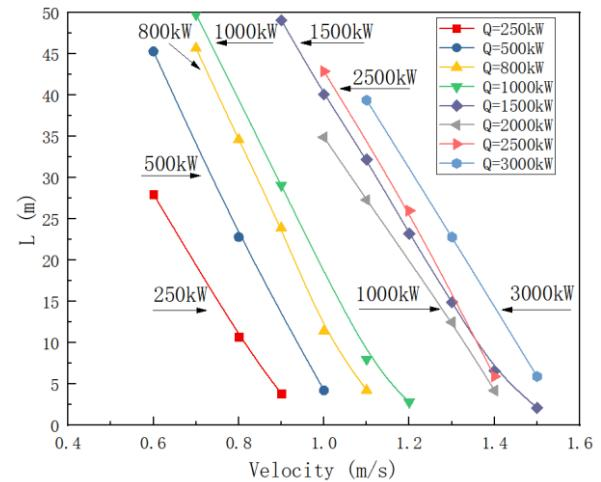
Fig. 3. The smoke back-layering length the utility tunnel with fire located at center line C.
