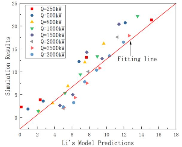
Fig. 8. The comparison between back-layering lengths of simulations results and Li's model predictions when fire source located at side A.
