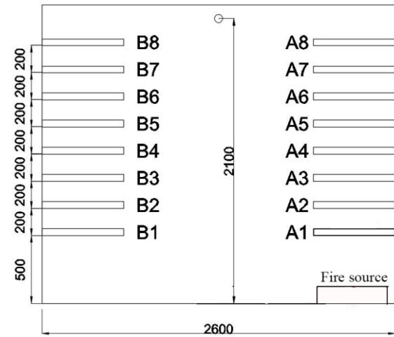
Fig. 2. Cross-sectional view of the utility tunnel with fire located at one side A.
