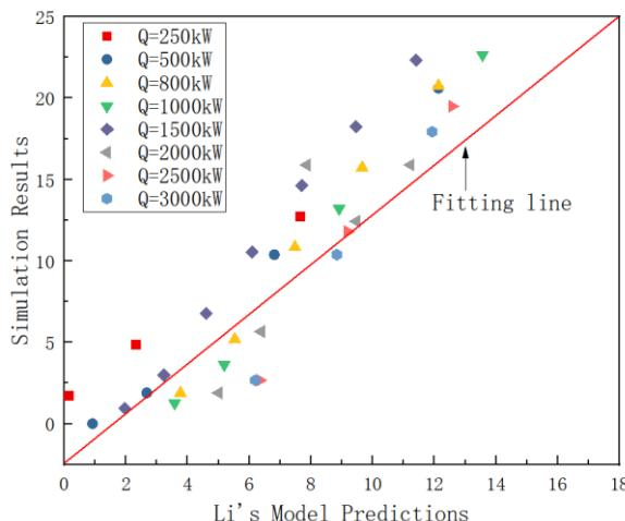
Fig. 9. The comparison between smoke back-layering length of simulation results and Li's model predictions when fire source located at center line C.
