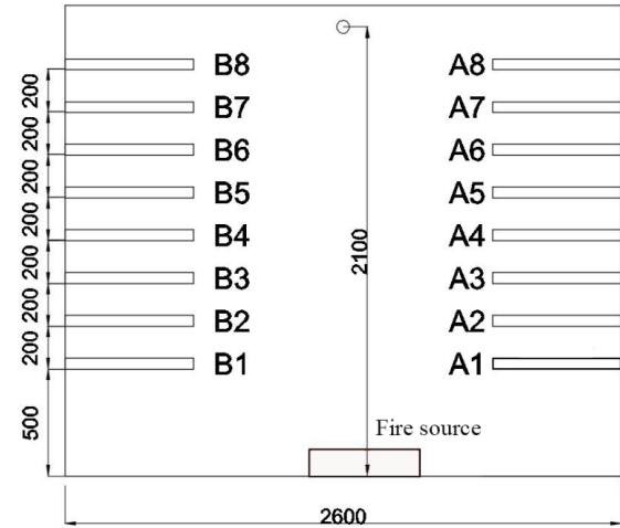
Fig. 1. Cross-sectional view of the utility tunnel with fire located at centerline C.
