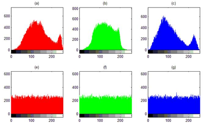
Fig. 4: Histograms of Baboon in red, green, and blue. Histograms of plain and cipher image are shown in row 1 and 2, respectively.
