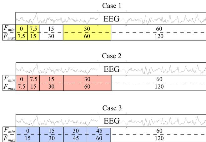
Fig. 7. Cutoff frequencies for the Multi-rate filter banks.
