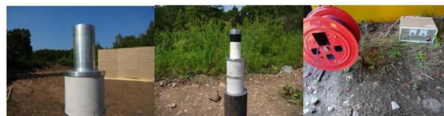
(a) Emplacing the warhead (b) Emplacing the detonator (c) Detonating the warhead
