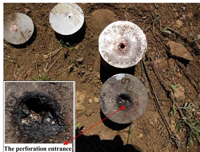
Fig.14. Damage effect of penetration.
