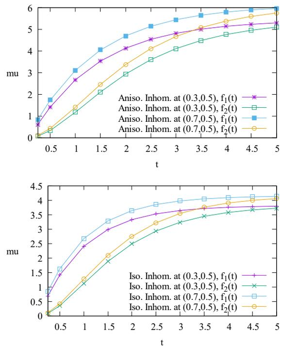
Fig. 6. Solutions  $\mu$  at  $(x_1, x_2) = (0.3, 0.5), (0.7, 0.5)$  for Case 3 (quadratically graded material) of Problem 2
