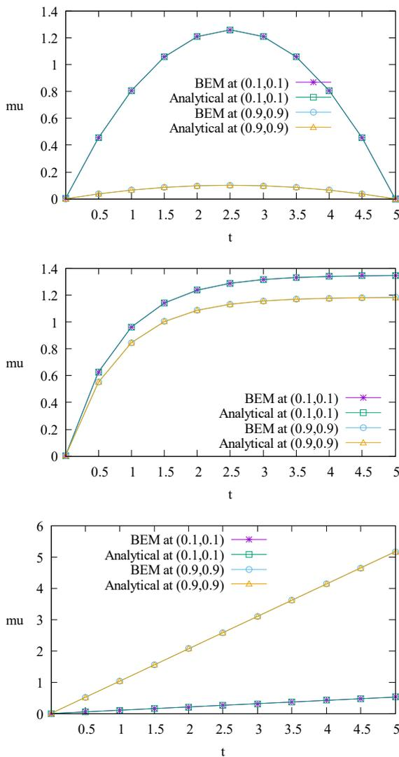
Fig. 2. Solutions  $\mu$  at some interior points  $(x_1, x_2)$  for the Case 1 (top), Case 2 (center) and Case 3 (bottom) of Problem 1
