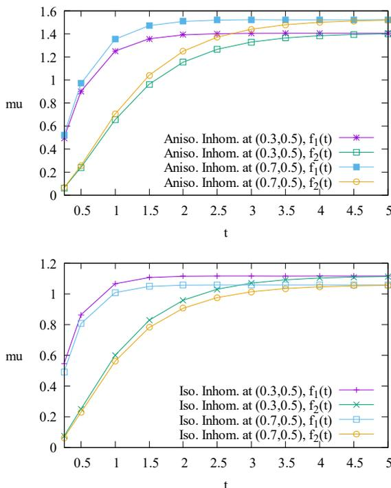
Fig. 5. Solutions  $\mu$  at  $(x_1, x_2) = (0.3, 0.5), (0.7, 0.5)$  for Case 2 (exponentially graded material) of Problem 2
