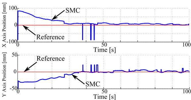
Fig. 18. Comparison analysis for tracking performance of the Sliding Mode Controller over prototype of Fig. 6 with a 30mm diameter ball
