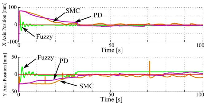
Fig. 24. Comparison analysis for tracking performance of the PID, Sliding Modes and Fuzzy controller over prototype of Fig. 6 with a 40mm diameter ball
