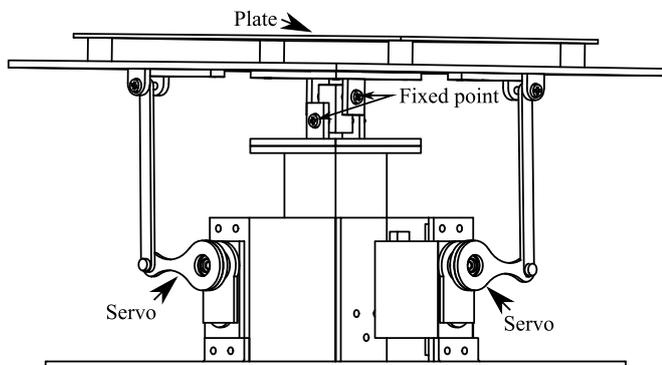
Fig. 3. Mechanical design of the Ball and Plate prototype system
