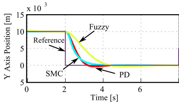
Fig. 16. Comparison analysis of PID, Sliding Modes and Fuzzy controller applied over the simulated Ball and Plate system for an impulse reference signal
