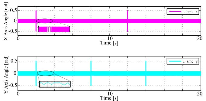
Fig. 10. Sliding Mode control signal of the simulated Ball and Plate for each axis
