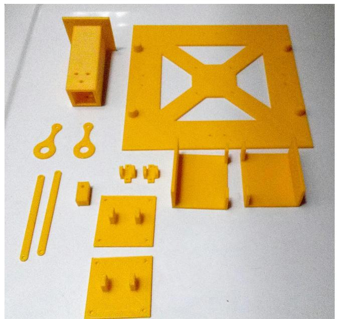
Fig. 5. 3D printed parts of the Ball and Plate final prototype
