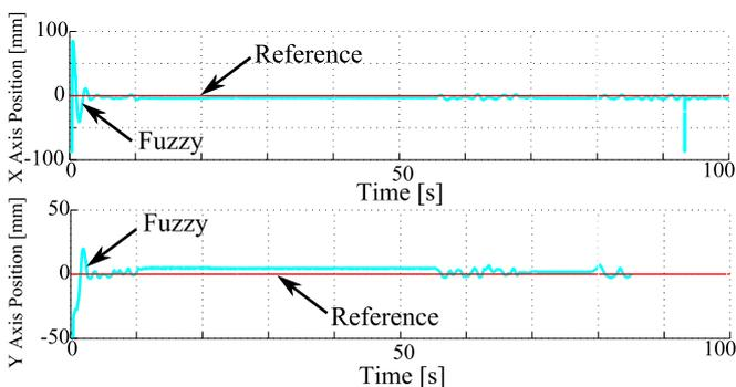
Fig. 19. Comparison analysis for tracking performance of the Fuzzy controller over prototype of Fig. 6 with a 30mm diameter ball
