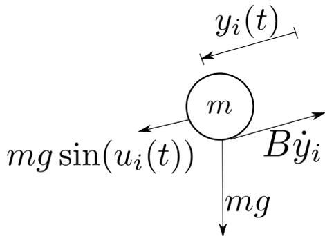
Fig. 2. Ball and plate free body diagram for  $i$ -axis
