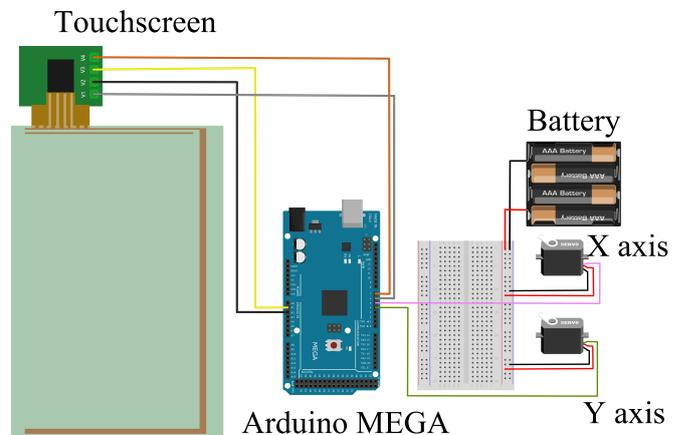
Fig. 4. Schematic diagram of the Ball and Plate prototype
