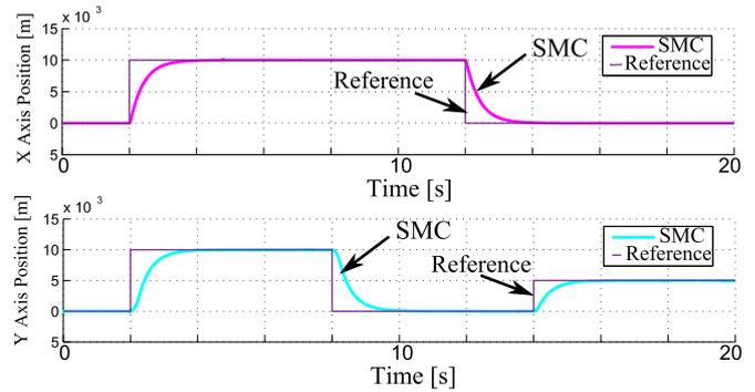
Fig. 9. Sliding Mode controller tracking performance of the simulated Ball and Plate system
