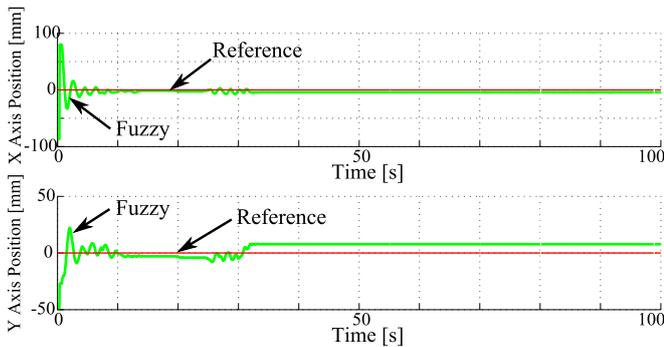
Fig. 23. Comparison analysis for tracking performance of the Fuzzy controller over prototype of Fig. 6 with a 40mm diameter ball
