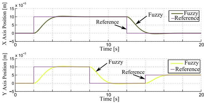
Fig. 12. Fuzzy controller tracking performance of the simulated Ball and Plate system
