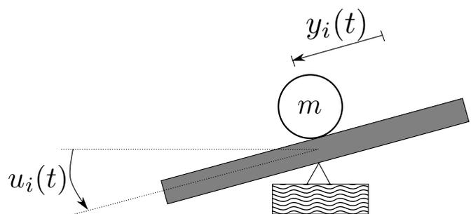
Fig. 1. Ball and plate schematic model for each  $i$ -axis
