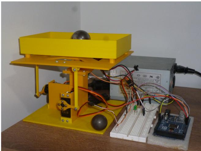
Fig. 6. Final prototype of the Ball and plate
