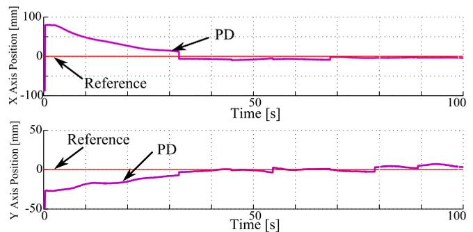
Fig. 21. Comparison analysis for tracking performance of the PID controller over prototype of Fig. 6 with a 40mm diameter ball
