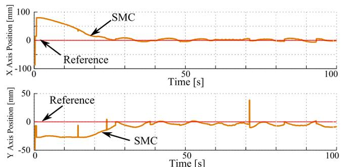
Fig. 22. Comparison analysis for tracking performance of the SMC controller over prototype of Fig. 6 with a 40mm diameter ball
