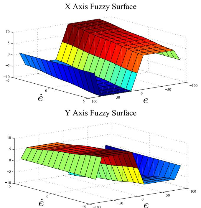
Fig. 11. Fuzzy surface for the simulated controller of the Ball and Plate system
