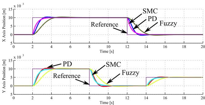
Fig. 14. Comparison analysis of PID, Sliding Modes and Fuzzy controller applied over the simulated Ball and Plate system
