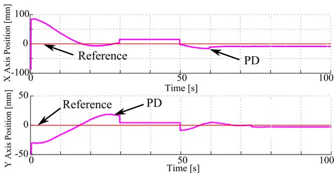
Fig. 17. Comparison analysis for tracking performance of the PID controller over prototype of Fig. 6 with a 30mm diameter ball
