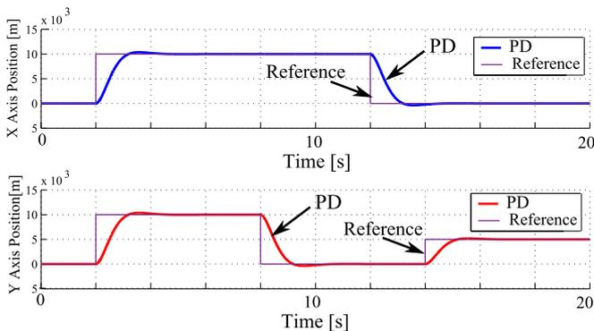
Fig. 7. PID controller tracking performance for each axis of the simulated Ball and Plate system
