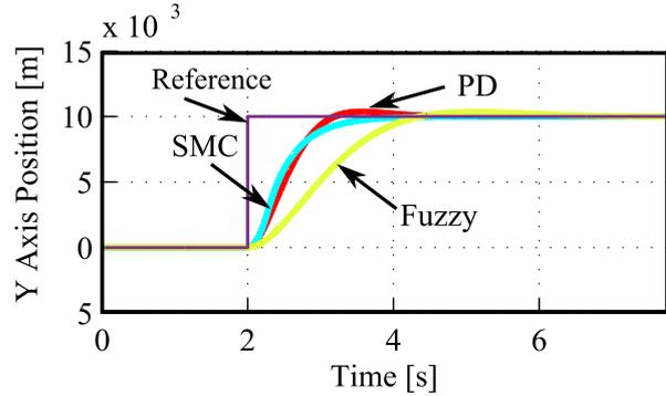
Fig. 15. Comparison analysis of PID, Sliding Modes and Fuzzy controller applied over the simulated Ball and Plate system for a step reference signal
