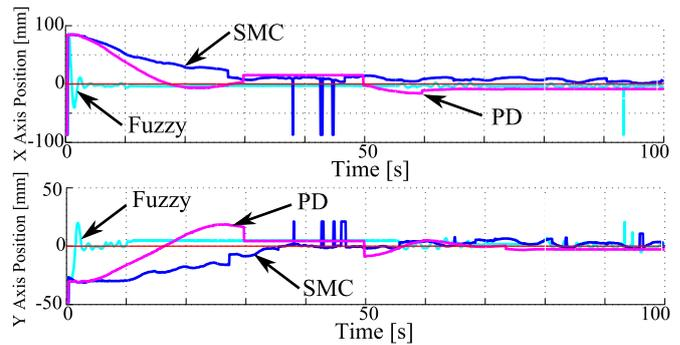
Fig. 20. Comparison analysis for tracking performance of the PID, Sliding Modes and Fuzzy controller over prototype of Fig. 6 with a 30mm diameter ball
