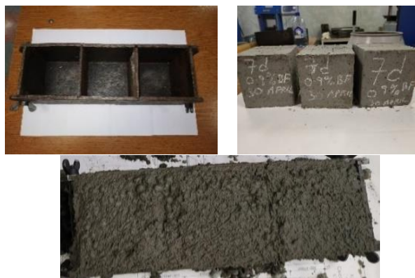
Fig. 2. Metallic cube mold.
