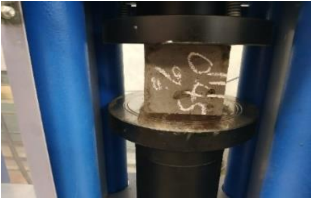
Fig. 3. Loading ECC cube specimen on the testing machine for compressive strength test.
