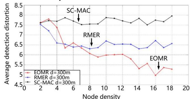
Fig. 9. Detection distortion of different node density areas at a distance of 300m from the sink node
