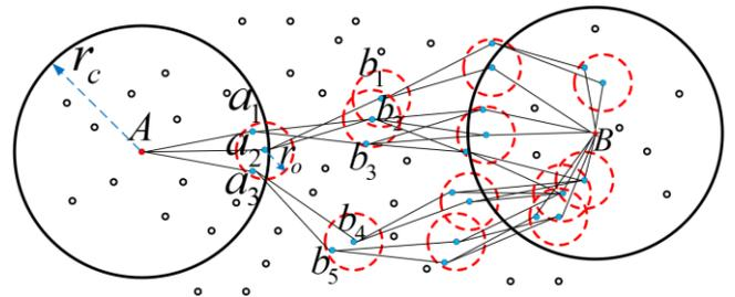
Fig. 5. The optimal routing path selection strategy based on FCS
