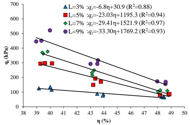
Fig. 14. Variation of split tensile strength with porosity for 30 days cure.
