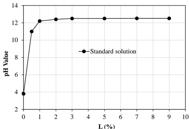
Fig. 3. Results of ICL tests for the soil-lime mixtures.
