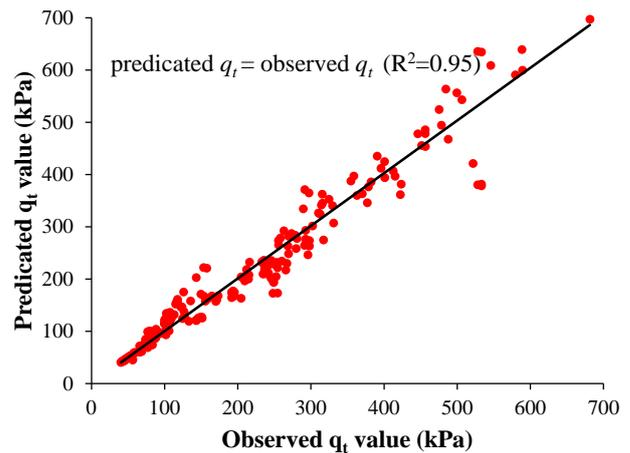
Fig. 23. Validation of estimate  $q_t$  for any cure time using  $\eta/L_v$  ratio.
