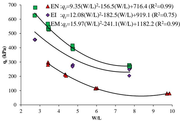
Fig. 12. Variation of split tensile strength with water/lime content ratio for 180 days cure.
