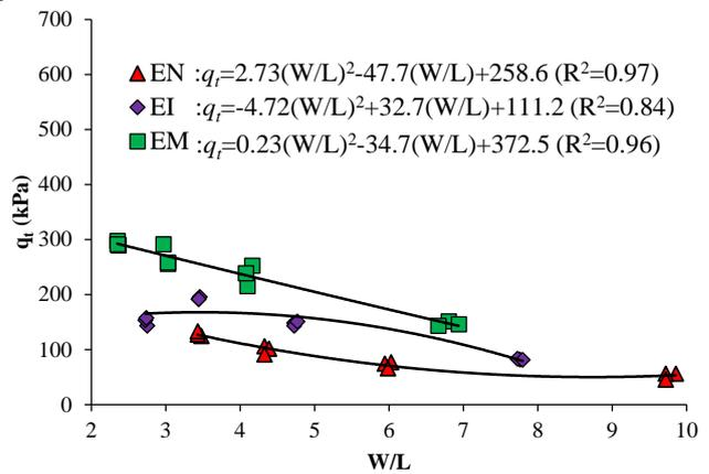
Fig. 9. Variation of split tensile strength with water/lime content ratio for 15 days cure.
