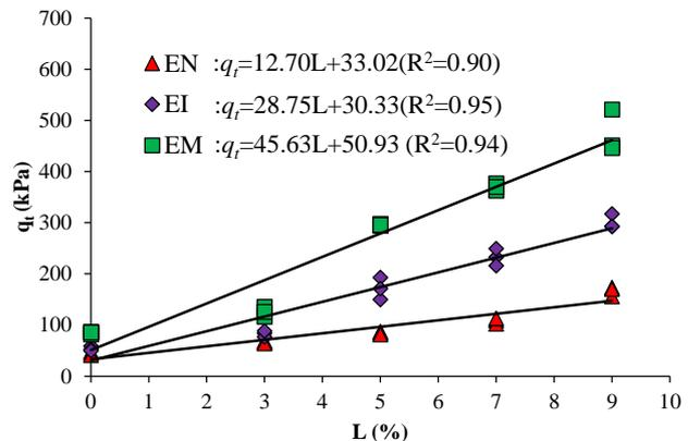
Fig. 6. Variation of split tensile strength with lime content for 30 days cure.
