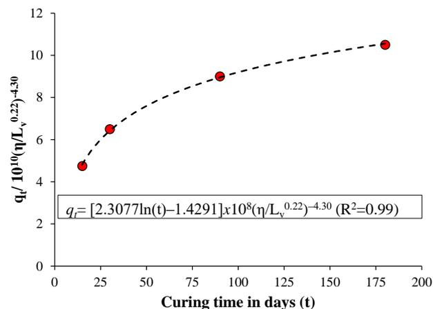
Fig. 22. Estimate  $q_t$  for any cure time using  $\eta/L_v$  ratio.
