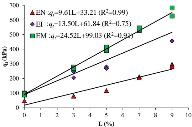
Fig. 8. Variation of split tensile strength with lime content for 180 days cure.
