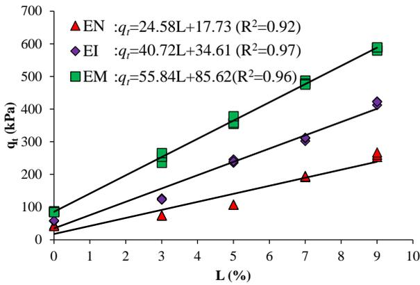
Fig. 7. Variation of split tensile strength with lime content for 90 days cure.
