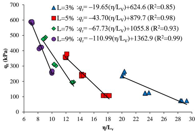
Fig. 19. Variation of split tensile strength with porosity/volumetric lime content ratio for 90 days cure.
