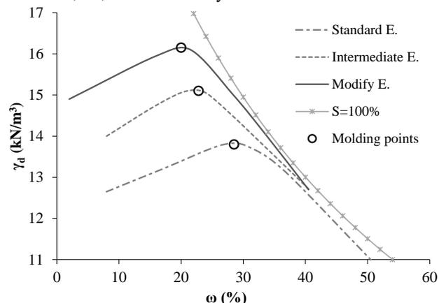
Fig. 4. Compaction curves and molding points.
