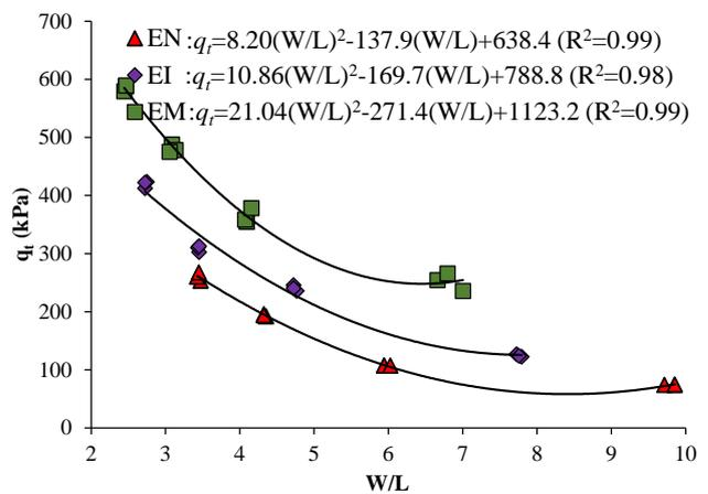
Fig. 11. Variation of split tensile strength with water/lime content ratio for 90 days cure.
