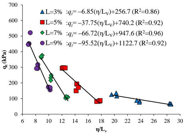
Fig. 18. Variation of split tensile strength with porosity/volumetric lime content ratio for 30 days cure.
