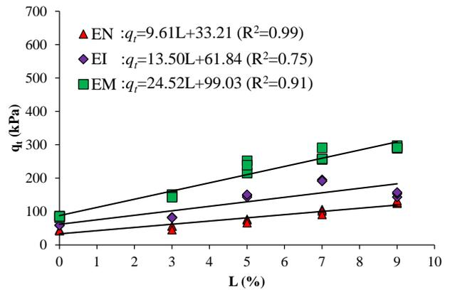
Fig. 5. Variation of split tensile strength with lime content for 15 days cure.
