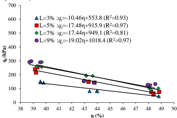
Fig. 13. Variation of split tensile strength with porosity for 15 days cure.
