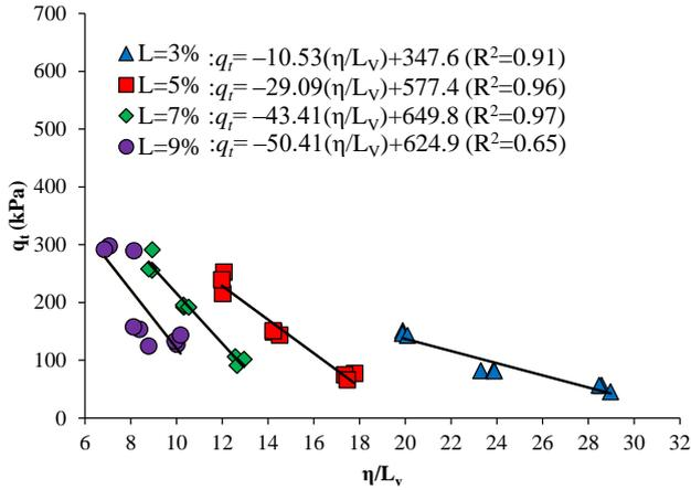
Fig. 17. Variation of split tensile strength with porosity/volumetric lime content ratio for 15 days cure.
