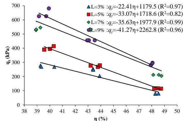
Fig. 16. Variation of split tensile strength with porosity for 180 days cure.
