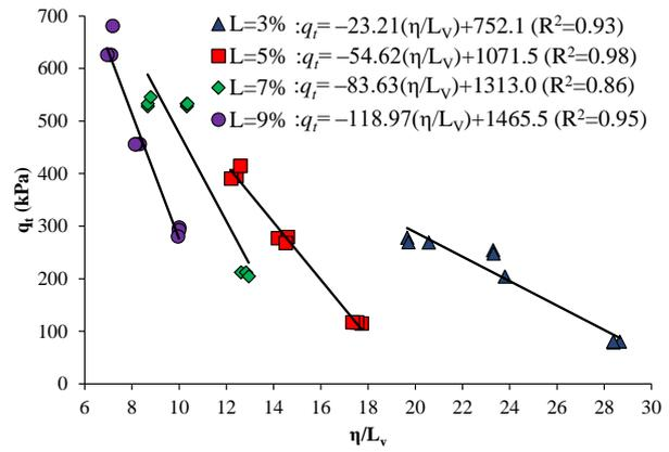
Fig. 20. Variation of split tensile strength with porosity/volumetric lime content ratio for 180 days cure.
