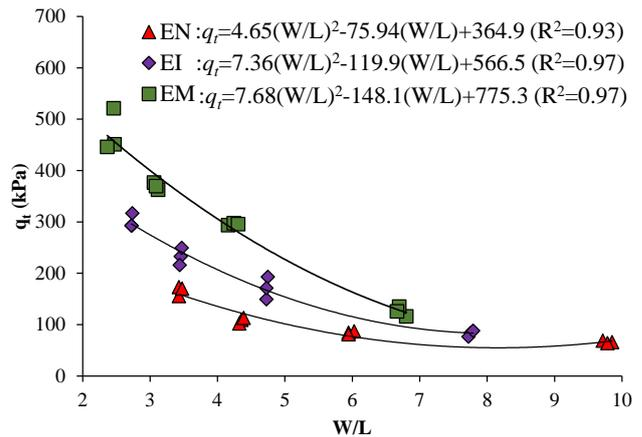
Fig. 10. Variation of split tensile strength with water/lime content ratio for 30 days cure.
