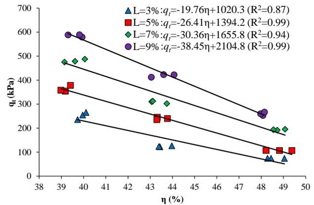
Fig. 15. Variation of split tensile strength with porosity for 90 days cure.
