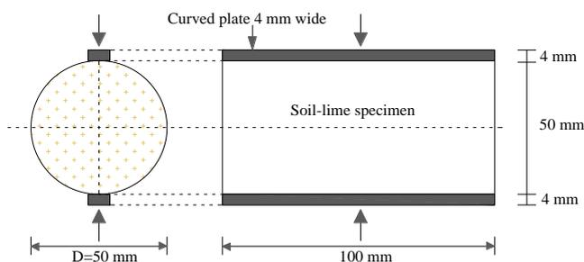
Fig. 1. Schematic sketch of specimen for split tensile test.
