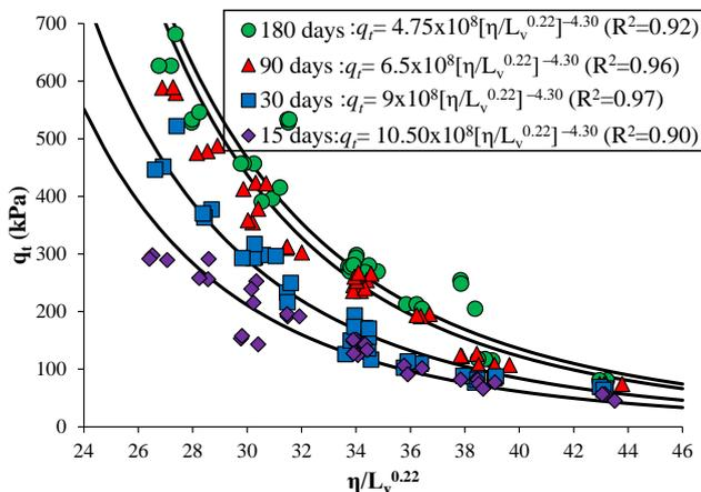
Fig. 21. Variation of Split tensile strength with porosity/volumetric lime content (using the exponent 0.22) ratio for 15, 30, 90, and 180 days cure.
